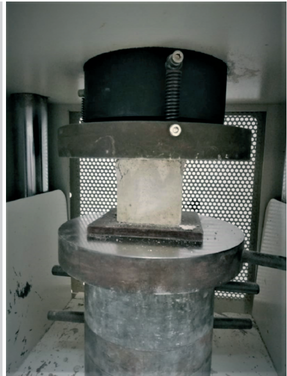
Figure 3. Setup of compression test
