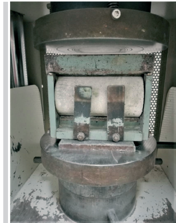
Figure 5. Setup of splitting tensile test
