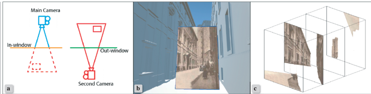
Figure 2. Window-camera positions for temporal windows (a), an image from the prototype (b), an example of image segmentation for parallax effect (c)
