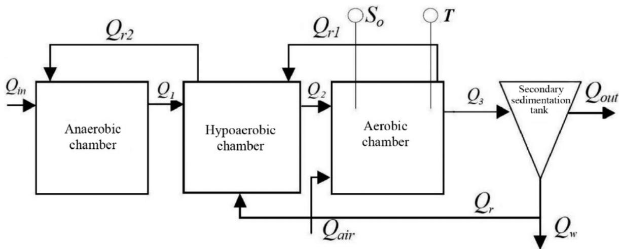
Figure 1. Biological reactor with the system of internal and external
