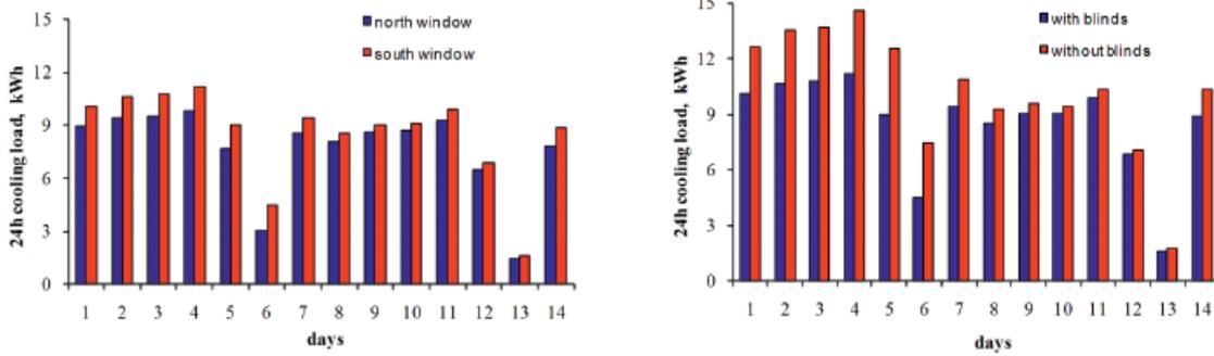
Figure 4. Comparison of 24 hours cooling demand for different windows location. a) north vs. south window exposition, b) south exposition, windows with and without blinds
