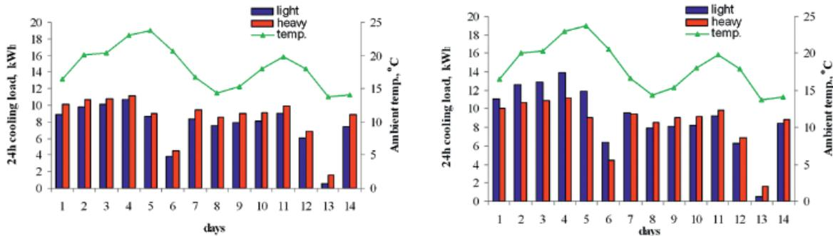
Figure 5. Comparison of 24 hours cooling demand for different building construction. a) windows with blinds, b) windows without blinds
