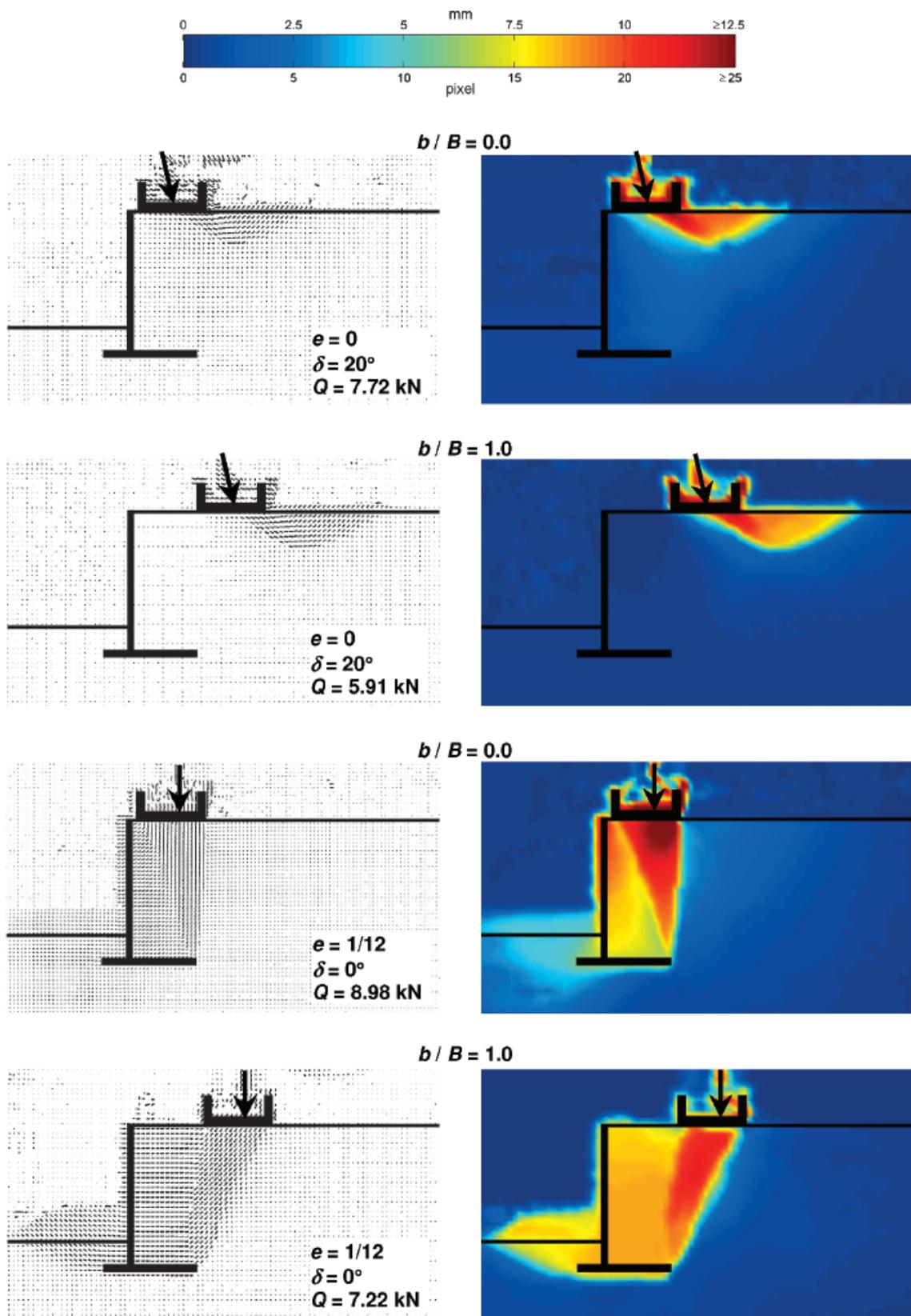
Figure 4. Trajectories and isoplots of displacement obtained by PIV technique in natural soil. Axial inclined and vertical eccentric loads
