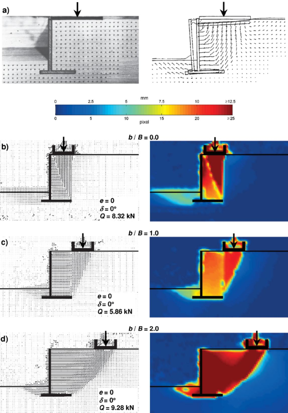
Figure 2. Trajectories and isoplots of displacement obtained by photogrammetry (a) and PIV technique (b) in natural soil. Axial and vertical loads
