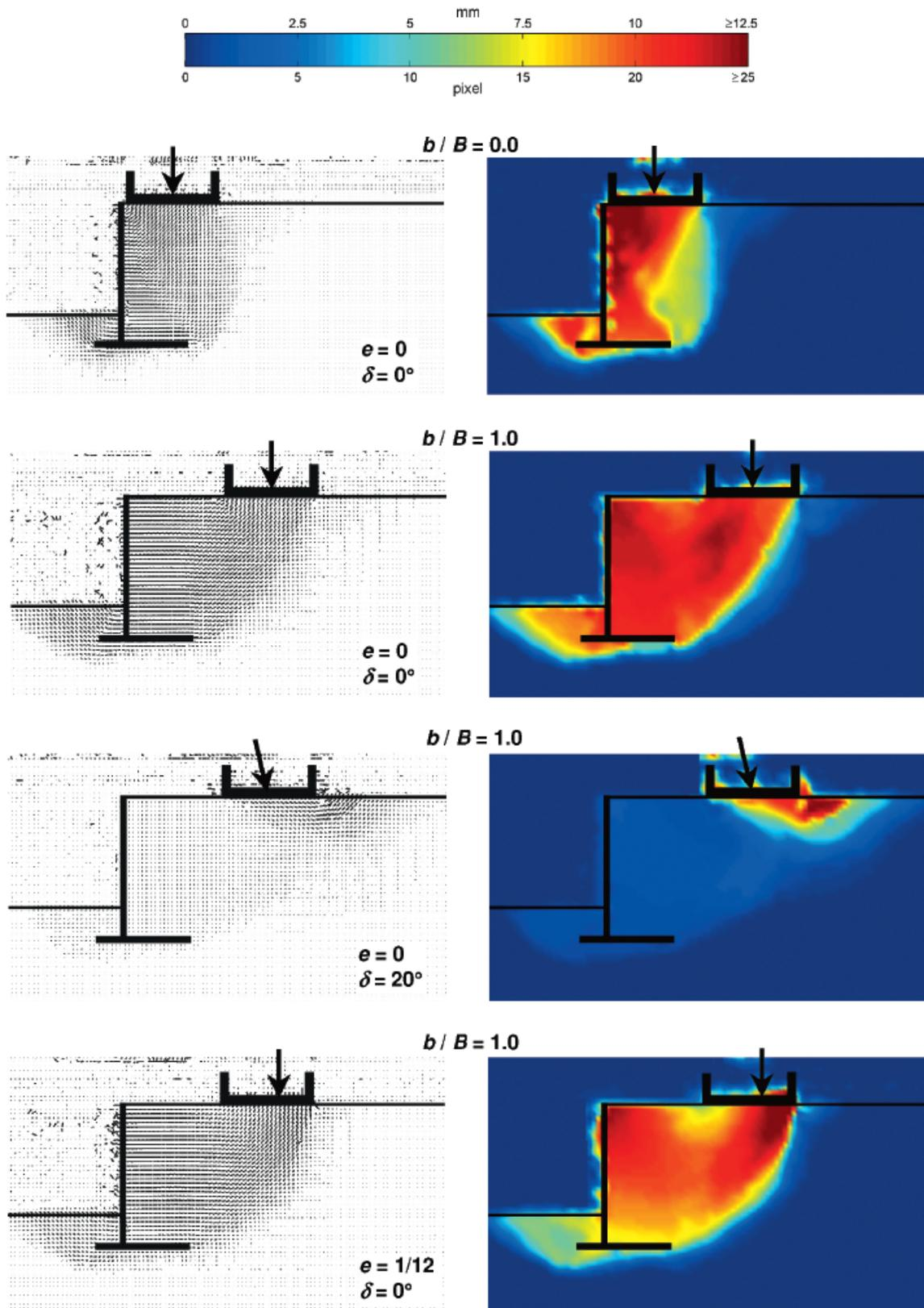
Figure 3. Trajectories and isoplots of displacement obtained by PIV technique in Taylor-Schnebelli analogue medium. Vertical axial or eccentric loads as well as axial inclined loads
