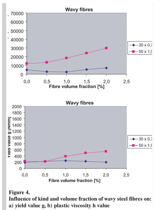
Condition of self-compacting was achieved for all considered wavy fibres in the whole range of variability of volume fraction. In case of the factor ( $F_F$ ), self-compacting limit for all wavy fibres was on the level 0.6. All tested hooked fibres except for the discussed above 64x0.80 fibres met self-compacting condition within the whole range of fibre reinforcement.
