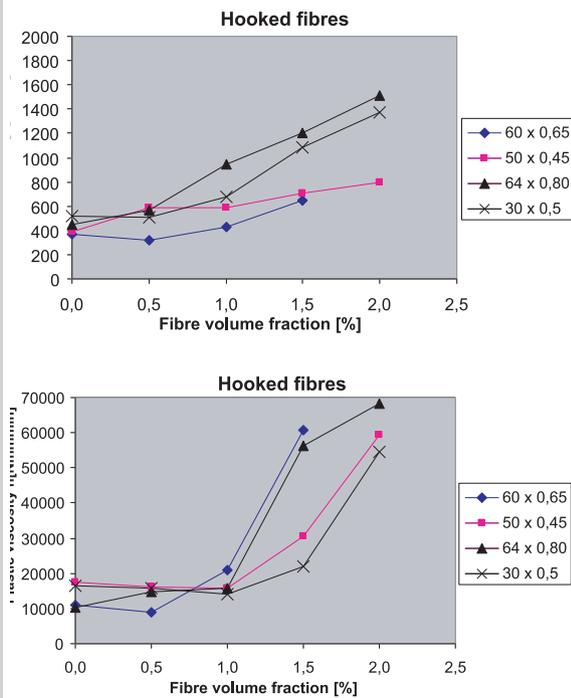
Figure 6. Influence of kind and volume fraction of hooked steel fibres on: a) yield value *g*, b) plastic viscosity *h* value
