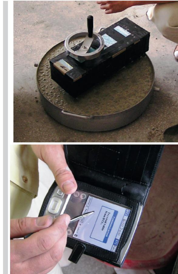
**Figure 1.** Rheometer BT-2 to determine rheological parameters of concrete mixes a) general view of the apparatus during the measuring procedure; b) readout and the verification of results of the rheometrical measurement
