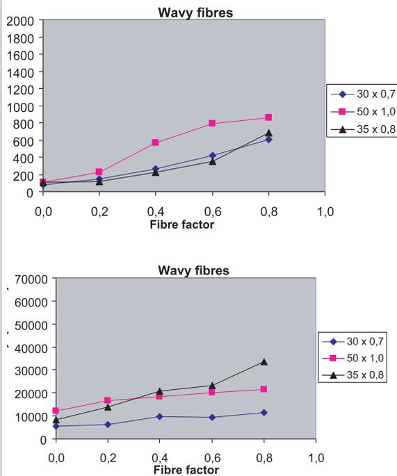
Figure 5. Influence of kind and fibre factor of wavy steel fibres on: a) yield value *g*, b) plastic viscosity *h* value
