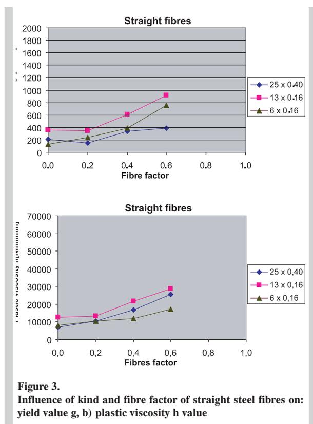
Addition of 6x0.16 fibres to the mixture resulted in the smallest increase of the  $h$  parameter. Thus the least worsening of the considered mixture workability was obtained. Similar results of examinations of self-compacting mixtures modified with straight fibres were obtained from research blocks I and II. Mixtures with the addition of 13x0.16 fibres started not to fulfil conditions for self-compacting mixtures sooner.
