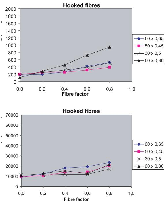
Figure 7. Influence of kind and fibre factor of hooked steel fibres on: a) yield value *g*, b) plastic viscosity *h* value
