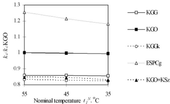
**Figure 4.** Relative  $k_c$  of thermomodernization of single-family building with optimal thermal insulation in function of nominal temperature of heating installation with floor heating and different heat sources
