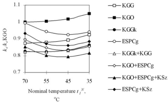
**Figure 3.** Relative total cost  $k_c$  of thermomodernization (windows, central heating installation, heat source) of multifamily building with  $U$ -value for walls according to requirements from year 2002 [7] in function of  $t_j^N$  for convection heater and different heat sources
