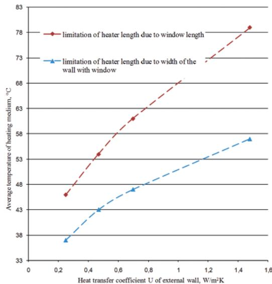
**Figure 1.** Relation between minimal (limited by the allowed length of the panel heater) average nominal temperature of heating medium and heat transfer coefficient  $U$  of external walls for typical multifamily building
