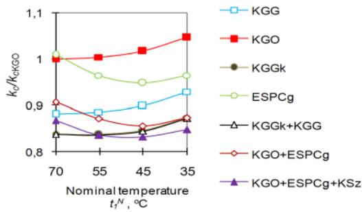
**Figure 2.** Relative average annual total cost ( $k_c/k_{c,KGO}$ ) of multifamily house thermomodernization (final thermal protection condition designate optimal thermal protection) in function of nominal supply temperature in installation with convective heaters presented for different heat sources
