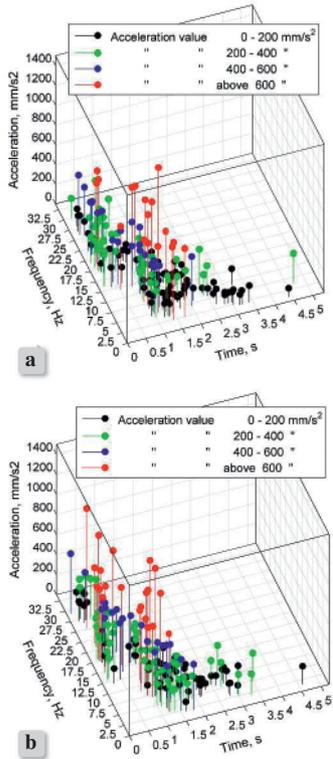
Figure 2. Diagrams of the local extremes of kinematic excitations, a) components X, b) components Y.
