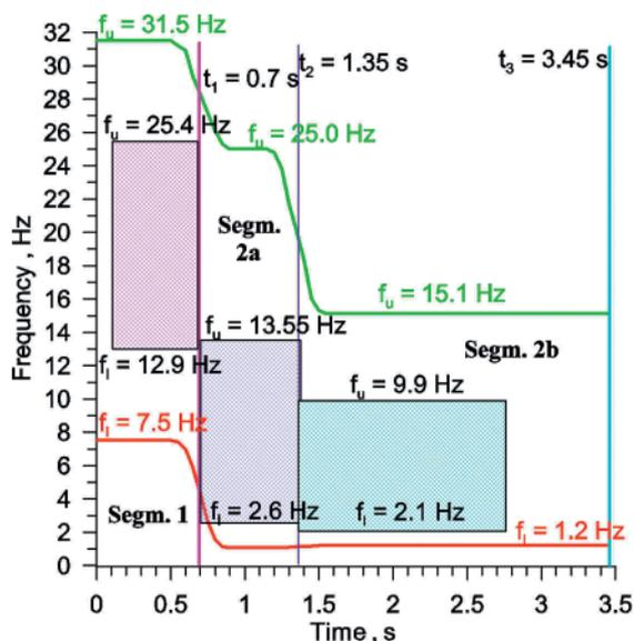
Figure 8. Time-frequency characteristics of kinematic excitations segments
