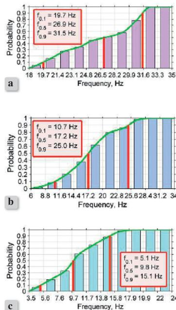
Figure 5. Frequencies in the upper bands of segments: a) No. 1, b) No. 2a, c) No. 2b
