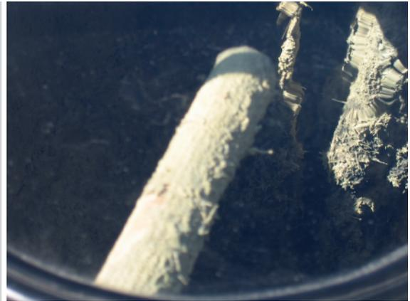
**Figure 8.** Deposition of elemental sulfur in a bioreactor during removal of sulfur compounds from biogas
