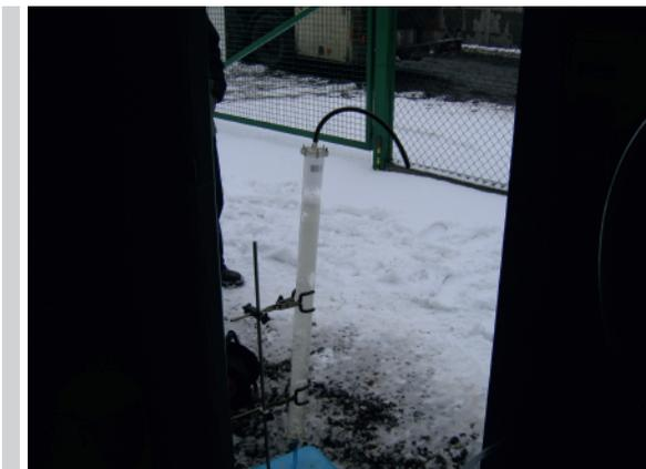
**Figure 7.** Research into biogas treatment, using a column filled with monoethanolamine. The tests were carried out at a municipal landfill site in Knurów, Poland
