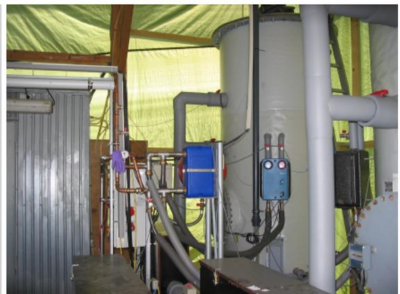
**Figure 10.** Installation used to remove hydrogen sulfide, using algae (Freising, branch of Technical University of Munich)
