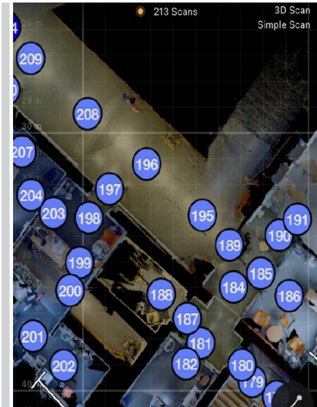
Figure 7. Map of photogrammetric scan positions of selected functional zones on the first floor of the school building in Gliwice. (own work)
