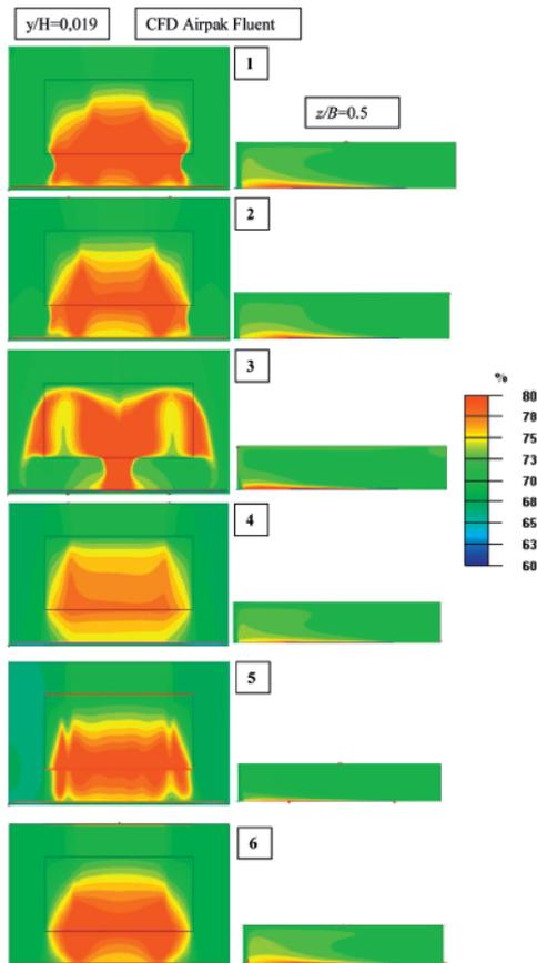
**Figure 10.** Maps of the relative humidity in the occupied zone of the swimming pool for various localizations of the outlets [7]:
