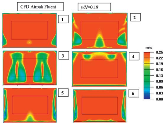
**Figure 9.** Maps of the average velocity in the occupied zone of the swimming pool for various localizations of the outlets [7]
