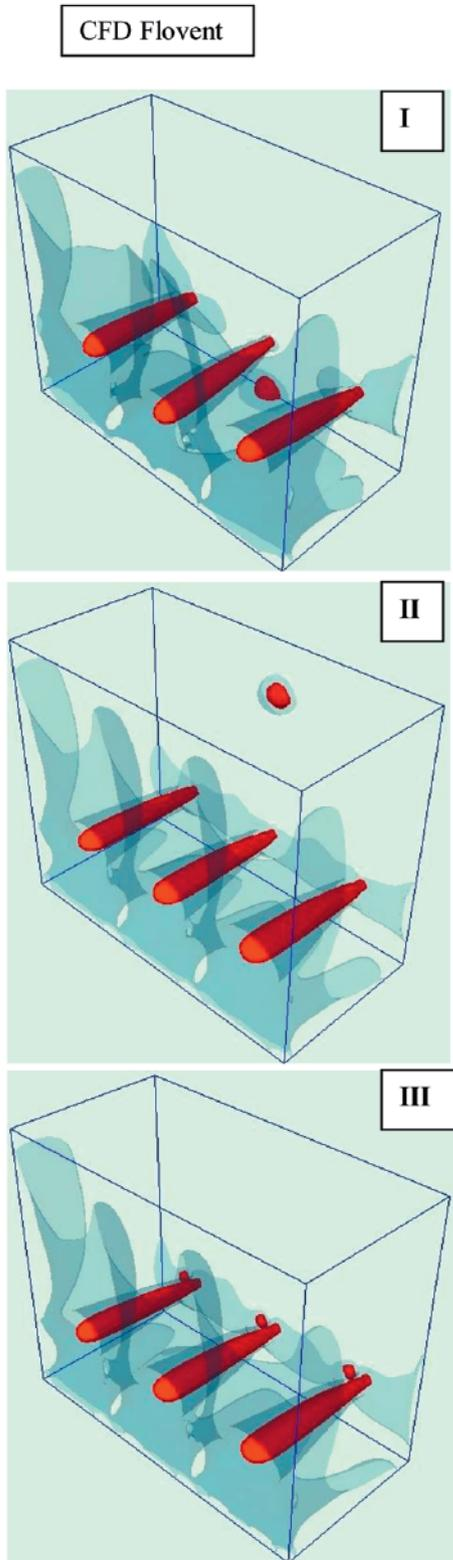
**Figure 2.** Distribution of the average velocity iso surfaces: 1 m/s and 0.35 m/s in the large hall for various heights of the outlets localization
