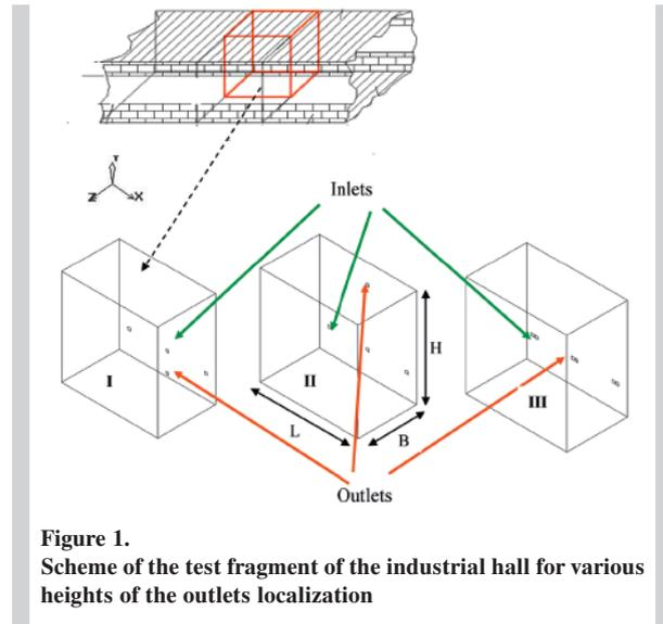
Figure 1. Scheme of the test fragment of the industrial hall for various heights of the outlets localization
