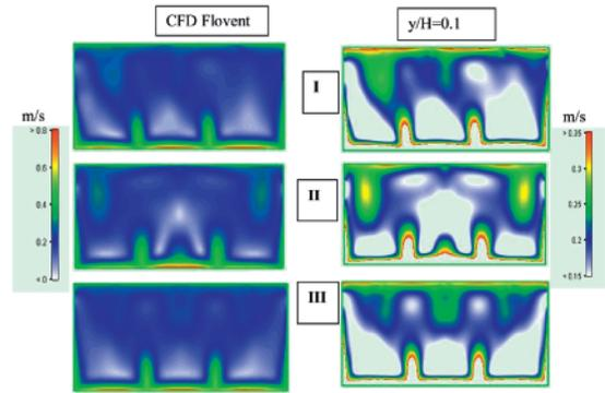
**Figure 3.** Distribution of the average velocity in the occupied zone of the large hall for various heights of the outlets localization: a) map of the average velocity b) isolines of the average velocity in the range 0.15-0.35 m/s
