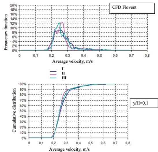
**Figure 4.** Comparison of the profiles of frequency function and cumulative distribution of average velocity in the occupied zone of the large hall for various heights of the outlets localization
