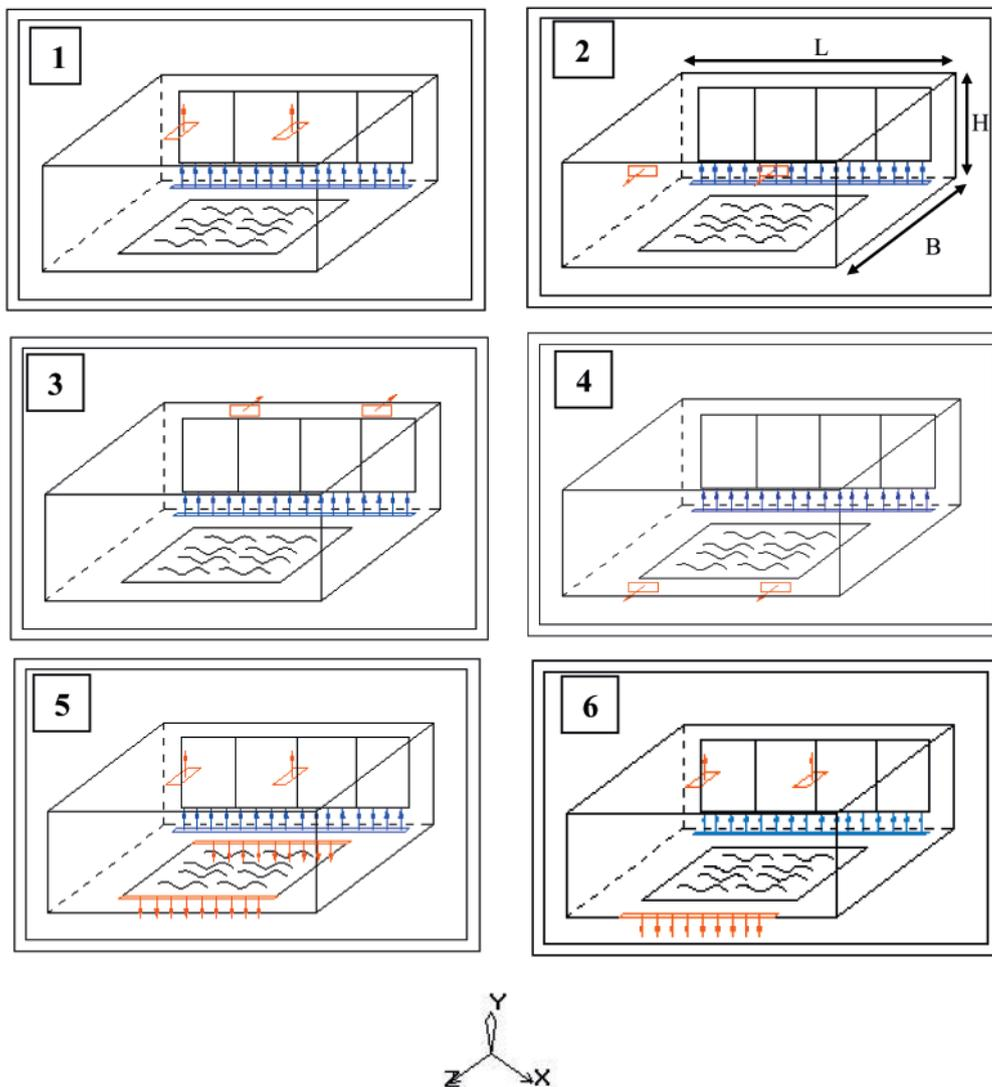
Figure 8. Schemes of the test swimming pool for the various localizations of the outlets
