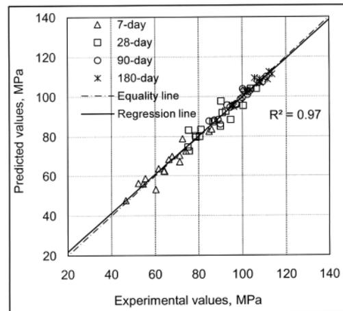
Figure 5. Relationship between experimental values and predicted values (using equation 2) of the compressive strength of concrete
