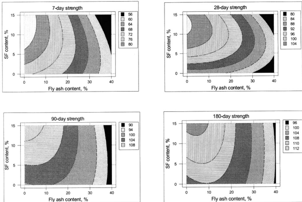
Figure 4. Predictive model for the compressive strength of concrete containing fly ash and SF (w/c 0.30) at various ages using equation 2
