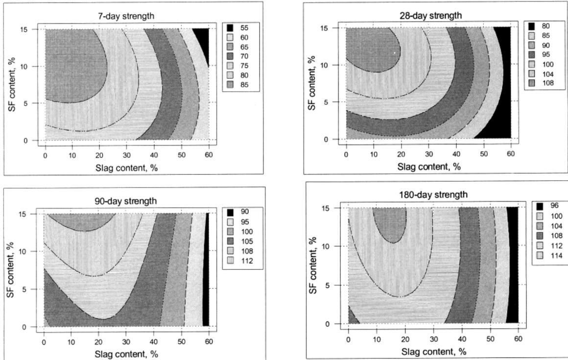
Figure 6. Predictive model for the compressive strength of concrete containing slag and SF (w/c 0.30) at various ages using equation 3
