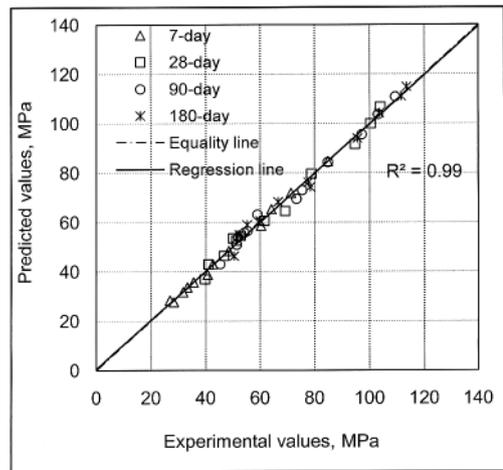
**Figure 9.** Relationship between experimental values and predicted values (using equation 4) of the compressive strength of concrete
