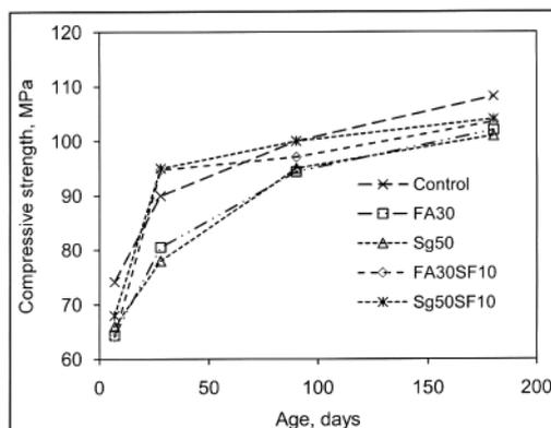
Figure 2. Compressive strength comparison of 30% FA and 50% Slag incorporating 10% SF (w/c 0.30)
