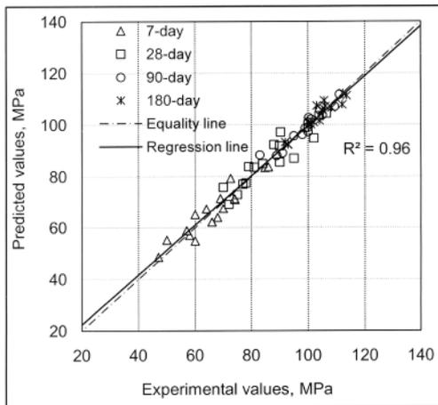
Figure 7. Relationship between experimental values and predicted values (using equation 3) of the compressive strength of concrete
