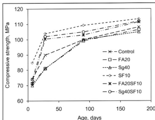
Figure 1. Compressive strength comparison of 20% FA and 40% Slag incorporating 10% SF (w/c 0.30)
