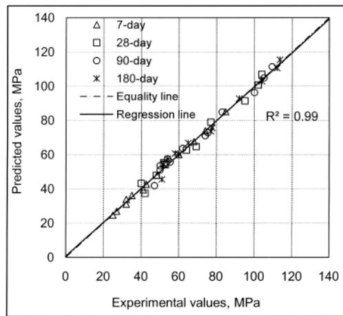
**Figure 11.** Relationship between experimental values and predicted values (using equation 5) of the compressive strength of concrete
