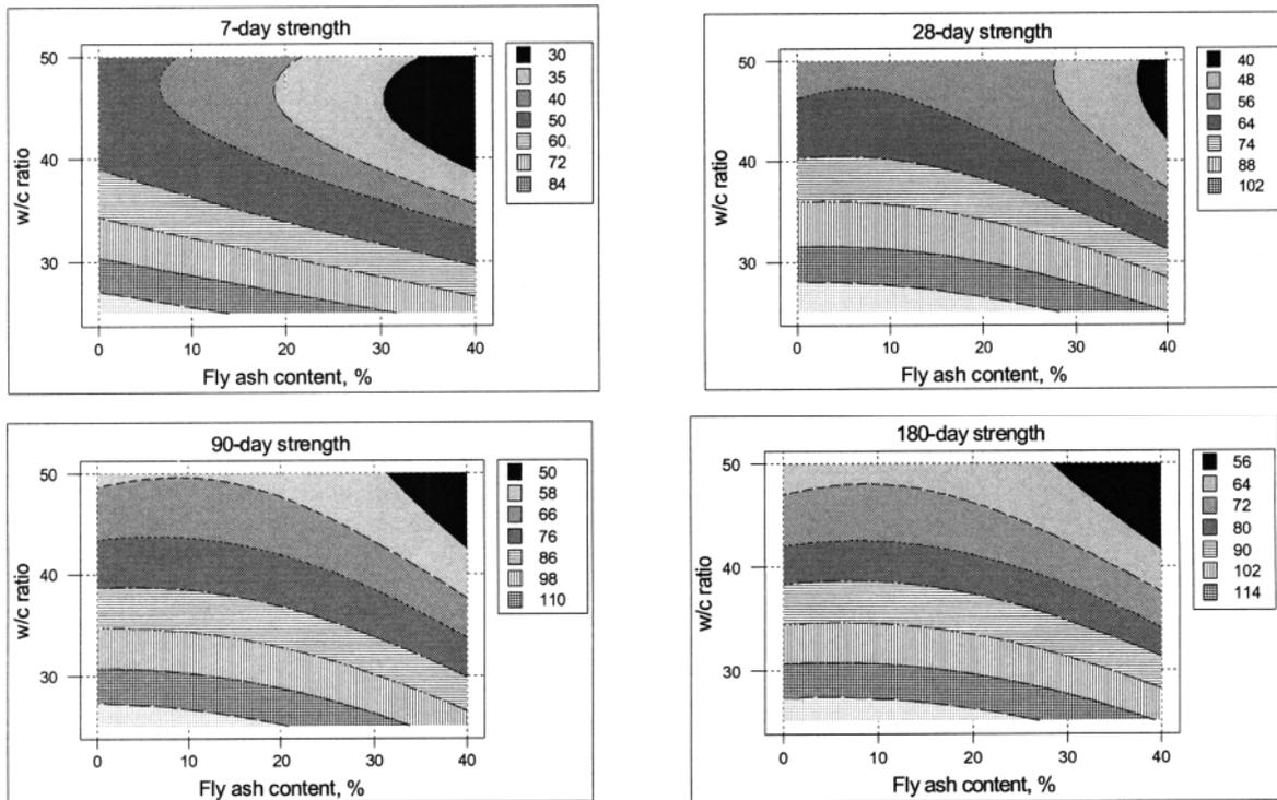
**Figure 8.** Predictive model for the compressive strength of concrete containing fly ash and 10% SF influenced by w/c ratio at various ages using equation 4.
