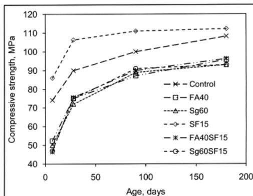
Figure 3. Compressive strength comparison of 40% FA and 60% Slag incorporating 15% SF (w/c 0.30)
