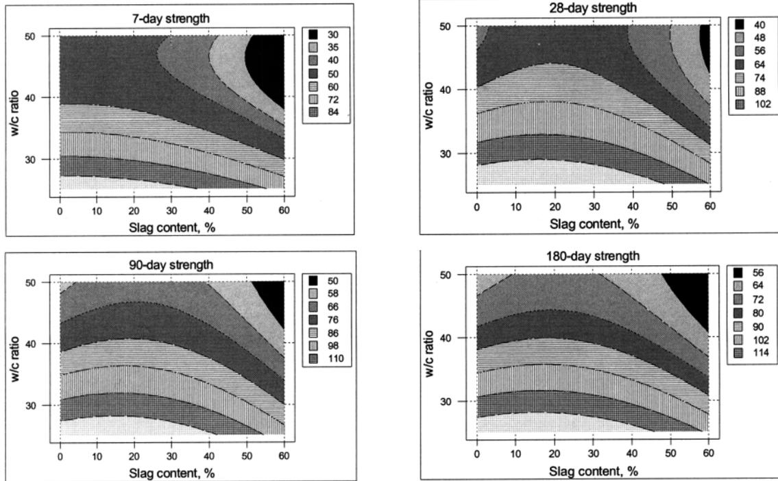
**Figure 10.** Predictive model for the compressive strength of concrete containing slag and 10% SF influenced by w/c ratio at various ages using equation 5
