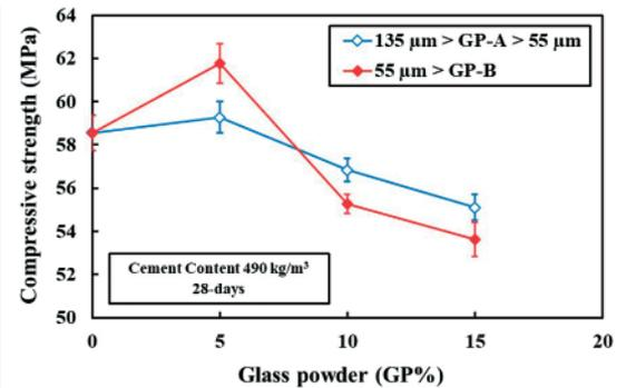
Figure 8. Short-term effect of GP-A and GP-B with various replacements on compressive strength development when cement content is relatively high (490 kg/m<sup>3</sup>)
