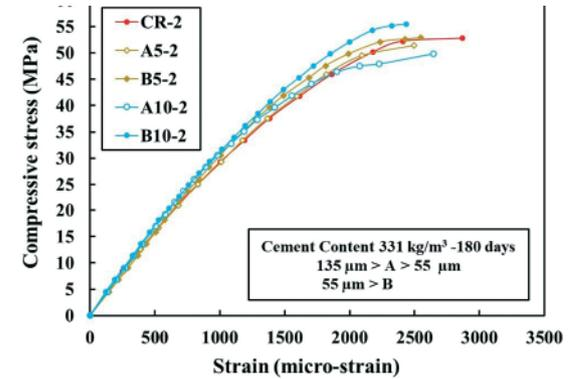
Figure 17. Effect of GP-A and GP-B with various replacements on non-linear stress-strain curves of concrete with a relatively low cement content (331 kg/m<sup>3</sup>)
