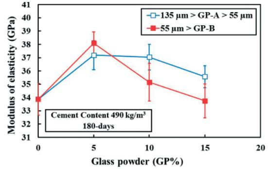
Figure 16. Long-term effect of GP-A and GP-B with various replacements on elastic modulus when cement content is relatively high (490 kg/m<sup>3</sup>)
