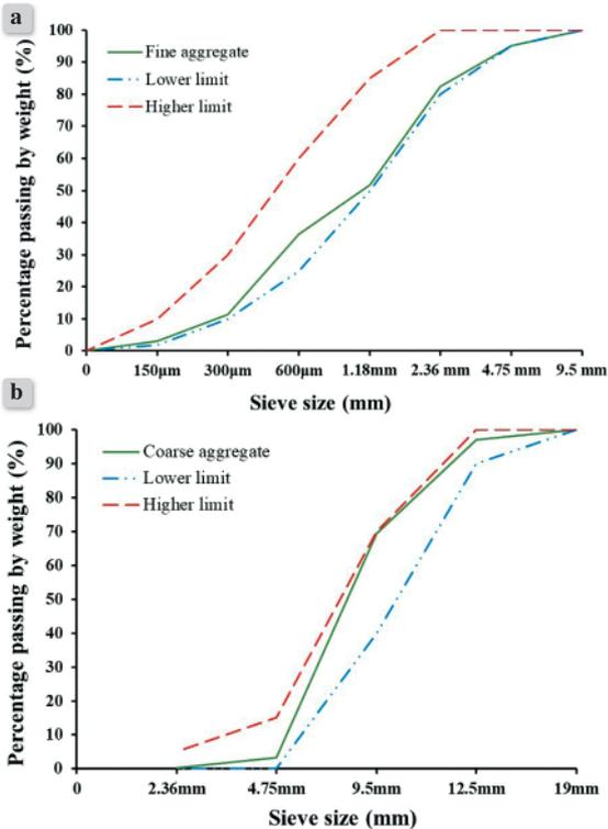
Figure 3. Grain size distribution for aggregates according to ASTM C33 limits. (a) sand and (b) gravel
