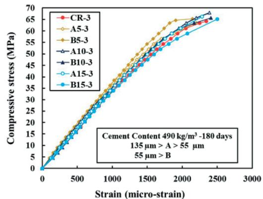
Figure 18. Effect of GP-A and GP-B with various replacements on non-linear stress-strain curves of concrete with a relatively high cement content (490 kg/m<sup>3</sup>)
