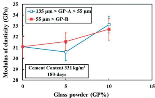
Figure 15. Long-term effect of GP-A and GP-B with various replacements on elastic modulus when cement content is relatively low (331 kg/m<sup>3</sup>)
