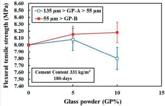
Figure 13. Long-term effect of GP-A and GP-B with various replacements on flexural tensile strength development when cement content is relatively low (331 kg/m<sup>3</sup>)
