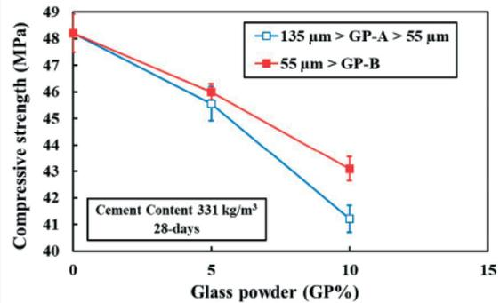
Figure 7. Short-term effect of GP-A and GP-B with various replacements on compressive strength development when cement content is relatively low (331 kg/m<sup>3</sup>)
