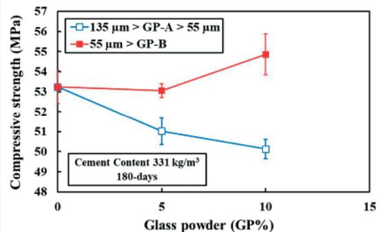
Figure 9. Long-term effect of GP-A and GP-B with various replacements on compressive strength development when cement content is relatively low (331 kg/m<sup>3</sup>)
