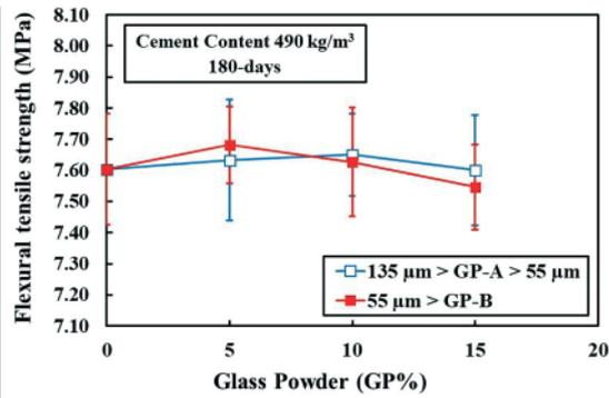
Figure 14. Long-term effect of GP-A and GP-B with various replacements on flexural tensile strength development when cement content is relatively high (490 kg/m<sup>3</sup>)
