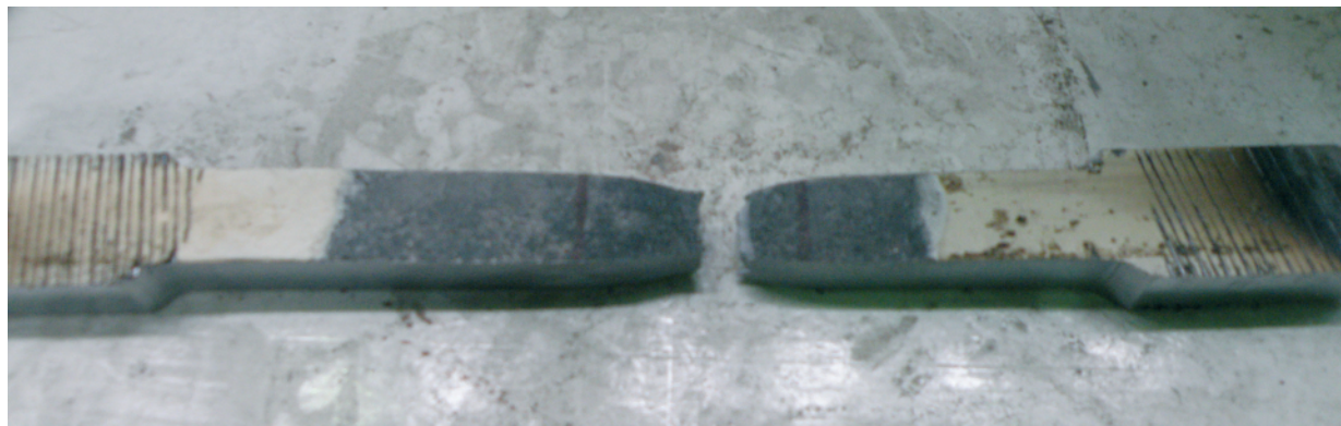
Figure 6. View of an exemplary 15 mm thick sample cut out of girder M 2.42 flange
