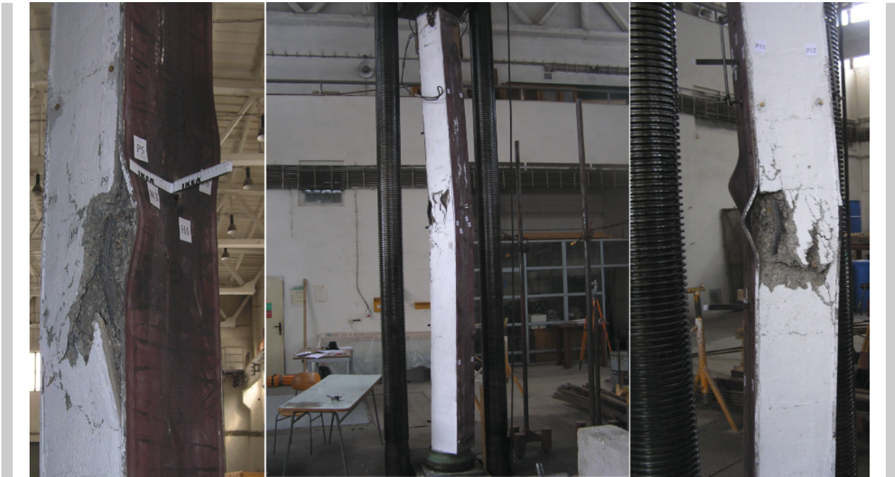
Figure 13. Failure of the SRC columns
