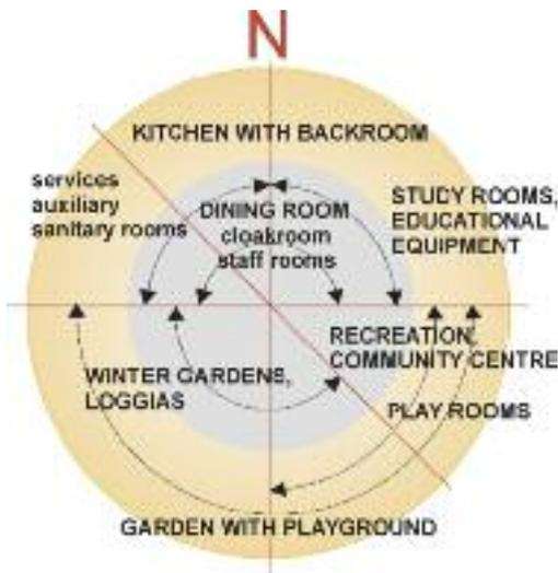
Figure 1. Author's schematic diagram of arrangement of rooms according to world's side-parts in functional building of nursery school. [6]
