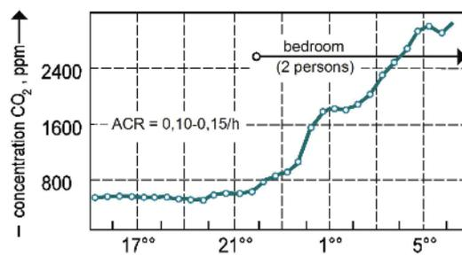
Figure 11. CO<sub>2</sub> concentration in bedroom with tight windows located on the 2<sup>nd</sup> floor level ( $t_e \cong 0^\circ\text{C}$ ,  $w \cong 0.3\text{m/s}$ )
