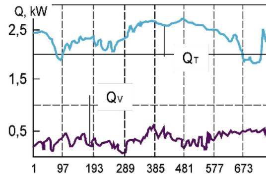
Figure 12. Comparison of an hourly total heat consumption ( $Q_T$ ) and heat consumption on ventilation ( $Q_V$ ) for flat (volume 167 m<sup>3</sup>) located on ground level of one of tested buildings (example for February)
