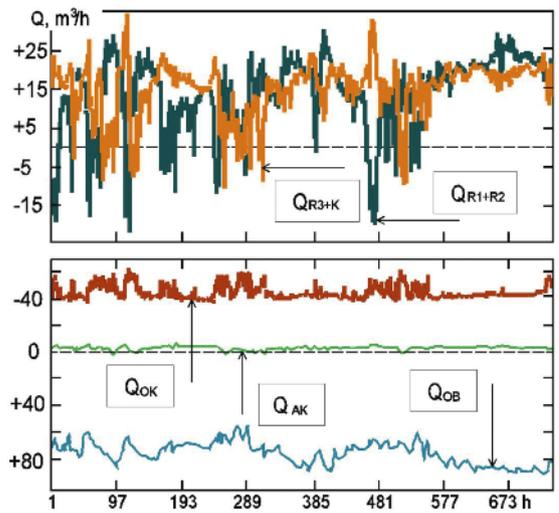
**Figure 15.** Hourly run variation of air flows in the flat located on the ground level of simulated building (the air leakage coefficients for all windows are 0.06 dm<sup>3</sup>/m<sup>2</sup>s at 1 Pa). Notations: QR<sub>1+R2</sub>, QR<sub>3+K</sub> – air inlets through gaps in windows, Q<sub>AR</sub> – as above but through gaps in the door (from the stairway), Q<sub>O</sub> – air outlets by natural ducts (from the kitchen – Q<sub>OK</sub> and bathroom – Q<sub>OB</sub>)
