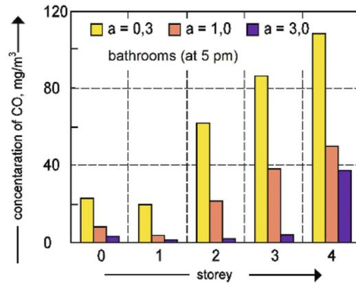
**Figure 18.** Dependence of carbon oxide concentration and air tightness building windows (the air leakage coefficients for windows a = 0.3; 1.0 and 3.0 m<sup>3</sup>/m<sup>2</sup>·h at 1 daPa)
