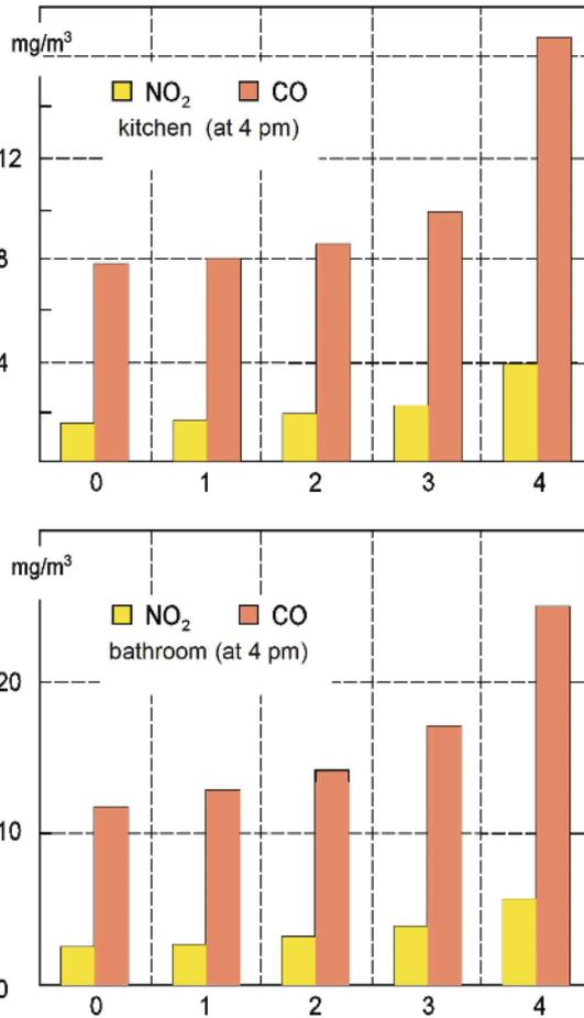
**Figure 17.** Concentration of NO<sub>2</sub> and CO inside kitchens and bathrooms located in several storeys and equipped with airtight windows (21 January) the air leakage coefficients for windows are 0.02 dm<sup>3</sup>/m<sup>2</sup>·s at 1 Pa or 0.3 m<sup>3</sup>/m<sup>2</sup>·h at 1 daPa
