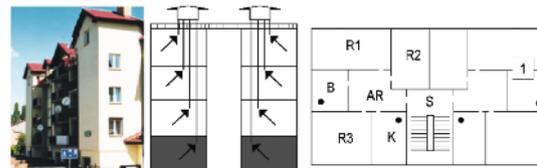
Figure 13. View and internal layout with selected section of simulated building. Notations: R1,2,3 – rooms, B – bathroom, K – kitchen, AR – anteroom, S – stairway, 1 – ventilation ducts
