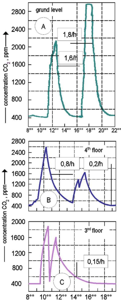
Figure 10. CO<sub>2</sub> concentration in three offices. Notations: A – the old windows and smoking, B – the tight windows and smoking, A,B – smoking (often), C – with tight windows
