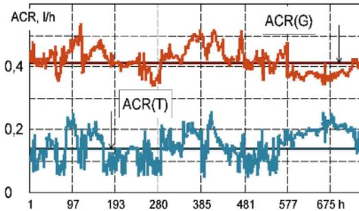
**Figure 14.** Run of ventilation rate in chosen flats of the building (the air leakage coefficients for windows are 0.06 dm<sup>3</sup>/m<sup>2</sup>s at 1 Pa). Notations: ACR(G) and ACR(T) – the air change in the flat located on the ground and the top storey
