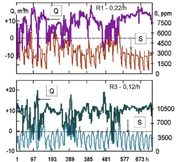
**Figure 16.** Changeability of air flows (Q) and CO<sub>2</sub> concentration (S) for two rooms (R1 and R3 as in Figure 20) and the leakage coefficients for all windows → 0.06 dm<sup>3</sup>/m<sup>2</sup>s at 1 Pa
