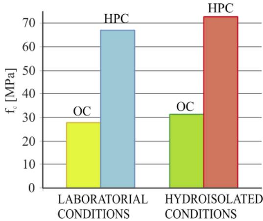
Figure 2. Twenty eight days compressive strength ( $f_c$ ) of concrete
