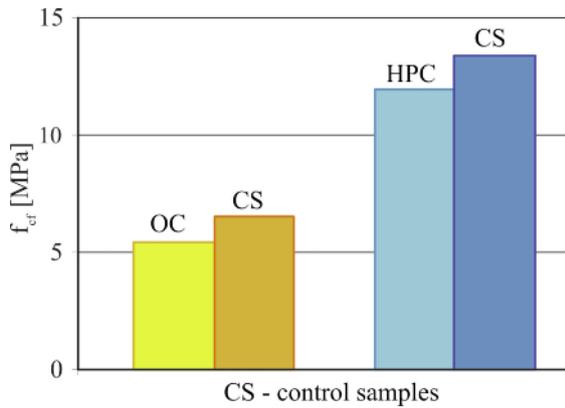
Figure 7. Tensile strength at bending ( $f_{ct}$ ) of concretes after 100 freeze-thaw cycles for laboratorial conditions
