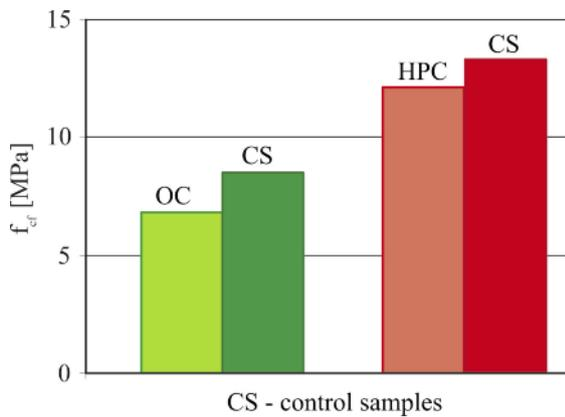
Figure 8. Tensile strength at bending ( $f_{ct}$ ) of concretes after 100 freeze-thaw cycles for hydroisolated conditions
