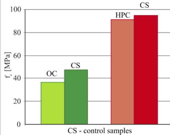
Figure 5. Compressive strength ( $f_c$ ) of concretes after 100 freeze-thaw cycles for hydroisolated conditions
