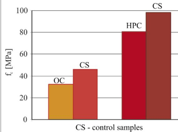
Figure 6. Compressive strength ( $f_c$ ) after 100 freeze-thaw cycles of concretes saturated with water to solid mass
