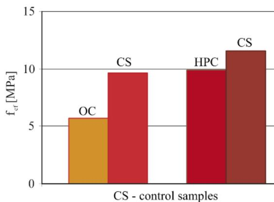
Figure 9. Tensile strength at bending ( $f_{ct}$ ) after 100 freeze-thaw cycles of concretes saturated with water to solid mass
