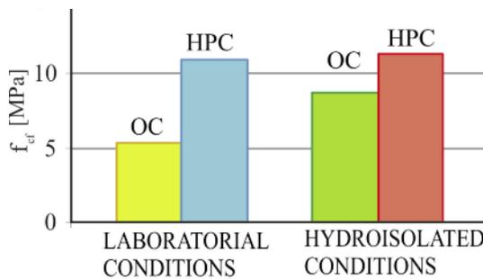
Figure 3. Twenty eight days tensile strength at bending ( $f_{ct}$ ) of concrete
