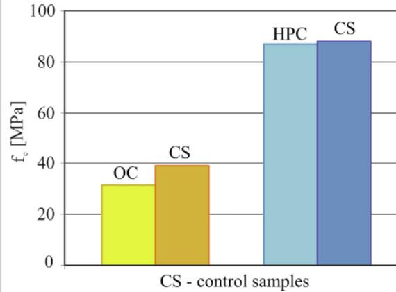
Figure 4. Compressive strength ( $f_c$ ) of concretes after 100 freeze-thaw cycles for laboratorial conditions
