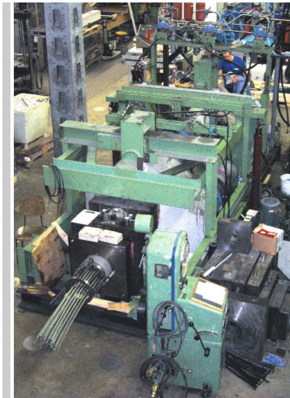
Figure 3. Test Set-up for the Fatigue and Tensile Test
