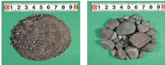
Figure 2. Recycled aggregates by heating and rubbing method
