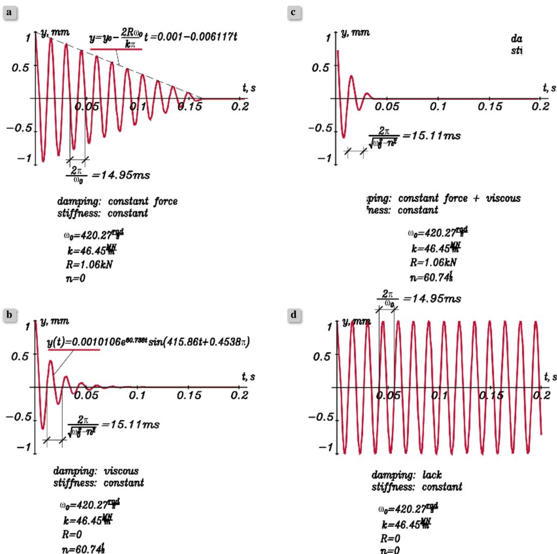
Figure 4. Results of analytical solutions of equation (18) at assumption  $y_{roz} = \infty$  a) solution for  $n=0$  and  $R \neq 0$ , b) solution for  $n \neq 0$  and  $R=0$ , c) solution for  $n \neq 0$  and  $R \neq 0$ , d) solution for  $n=0$  and  $R=0$
