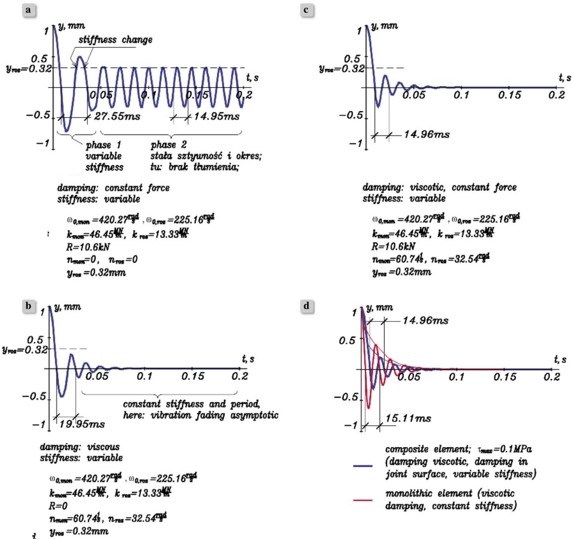
Figure 5. Numerical solution of equation (15) with initial conditions (33) on the assumption that  $y_{roz}=0.32$  mm, a) solution for  $n=0$  and  $R\neq 0$ , b) solution for  $n\neq 0$  and  $R=0$ , c) solution for  $n\neq 0$  and  $R\neq 0$ , d) comparison of solution in Fig. 4b (vibrations of monolithic structure) with solution of the equation in Fig. 5c (vibrations of composite structure)
