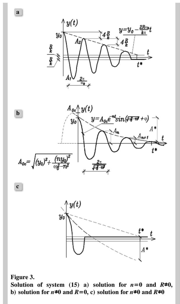
Figure 3. Solution of system (15) a) solution for  $n=0$  and  $R \neq 0$ , b) solution for  $n \neq 0$  and  $R=0$ , c) solution for  $n \neq 0$  and  $R \neq 0$
