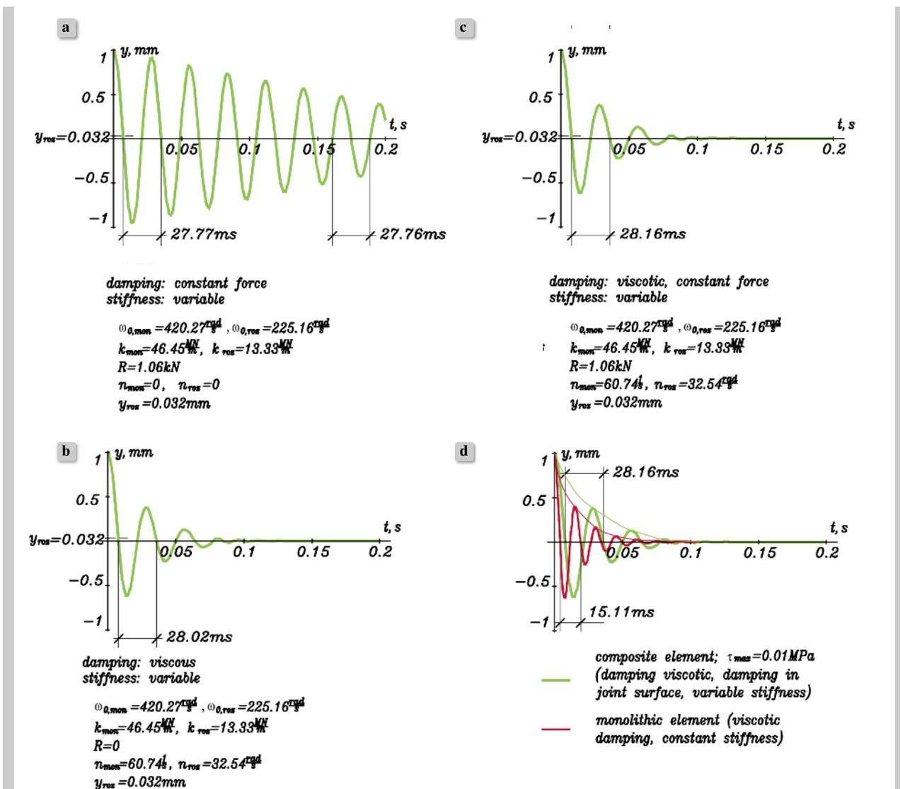
Figure 6. Numerical solution of equation (15) with initial conditions (33) on the assumption that  $y_{roz}=0.032\text{ mm}$ , a) solution for  $n=0$  and  $R\neq 0$ , b) solution for  $n\neq 0$  and  $R=0$ , c) solution for  $n\neq 0$  and  $R\neq 0$ , d) comparison of solution of equation (16) at  $n\neq 0$  and  $R\neq 0$  (vibrations of composite structure) with solution of equation in Fig. 4b (vibrations of monolithic structure)
