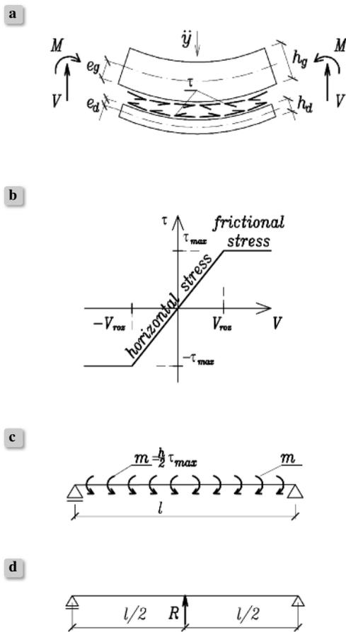
**Figure 1.** Assumptions of the model of vibrations damping a) frictional stress in joint surface b) horizontal stress ( $\tau$ ) and frictional stress ( $\tau_{max}$ ) as a function of transverse force c) frictional stress interaction as a uniformly distributed bending moment  $m$ , d) damping force  $R$  equivalent to frictional stresses interaction
