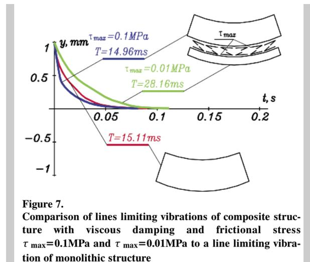
Figure 7. Comparison of lines limiting vibrations of composite structure with viscous damping and frictional stress  $\tau_{max}=0.1\text{MPa}$  and  $\tau_{max}=0.01\text{MPa}$  to a line limiting vibration of monolithic structure
