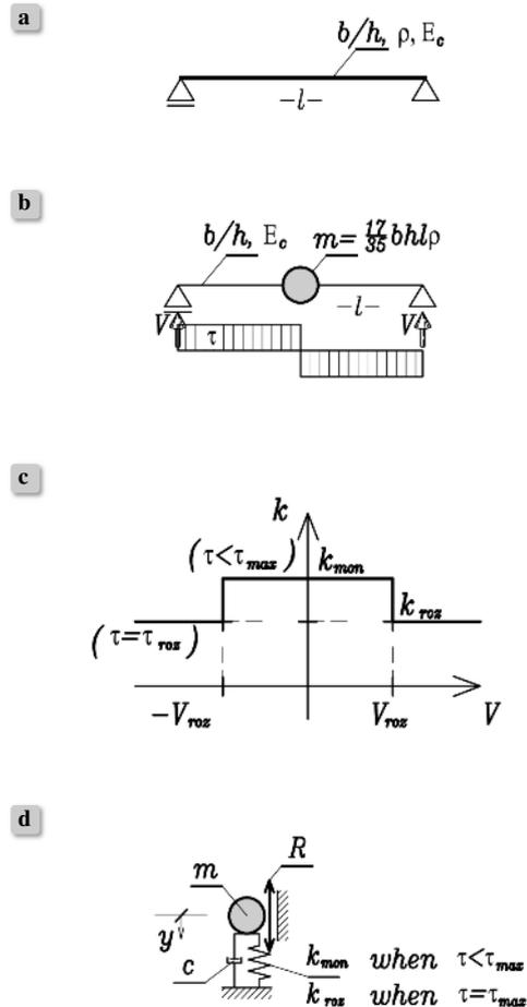
**Figure 2.** a) analysed system, b) substitute system, c) discretely variable stiffness of the system in relation to value of transverse force, d) damping elements in the system
