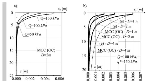
Figure 8. a) Settlement distribution under the foundation centre  $D=2m$ , b) Settlement distribution (to a depth of the subsoil model) for MCC (OC) and (e) models
