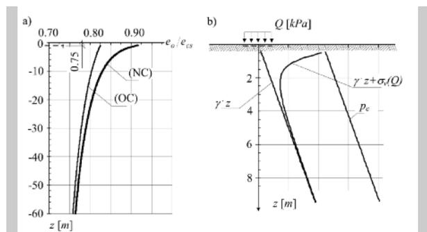
**Figure 6.** a) State (1) matrixes for the subsoil (NC) and (OC) obtained for the MCC (NC) and MCC (OC) models, b) the subsoil pre-consolidated for whole range of the loading value
