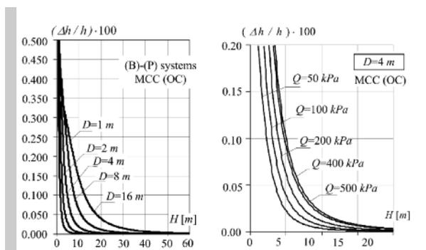
Figure 7. a) Function (4) – diagrams for different foundations  $D_i$ , b) Function (4.25) sensitivity to loading  $Q$  variations
