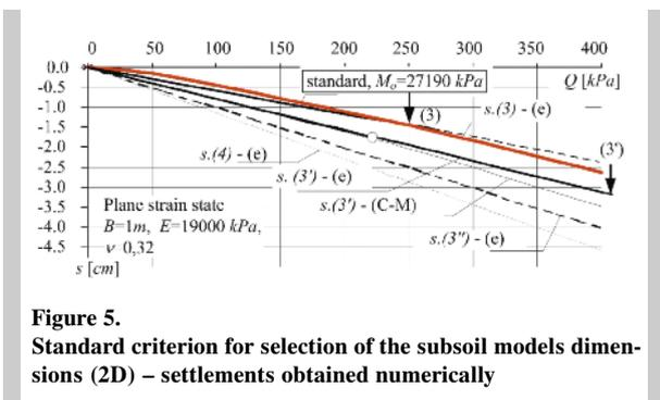
**Figure 5.** Standard criterion for selection of the subsoil models dimensions (2D) – settlements obtained numerically
