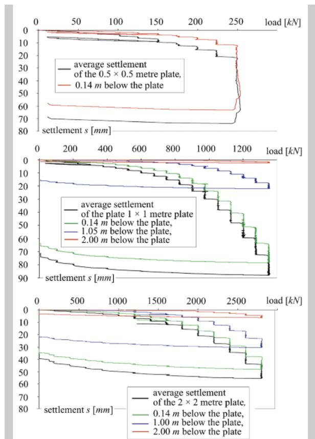
Figure 3. Experimental relations load-settlement for clay till [12]
