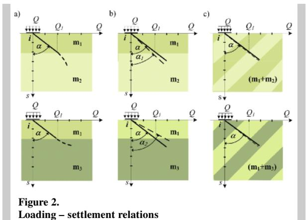
Figure 2a presents two “smoothed” dependencies load-settlement, hypothetically obtained in the in situ tests in bedded subsoils of different layers rigidity. Possibility of the same, initial system response to load expressed by angle  $\alpha$ . It is a result of linear-elastic, in initial phase, behaviour of soil medium.
