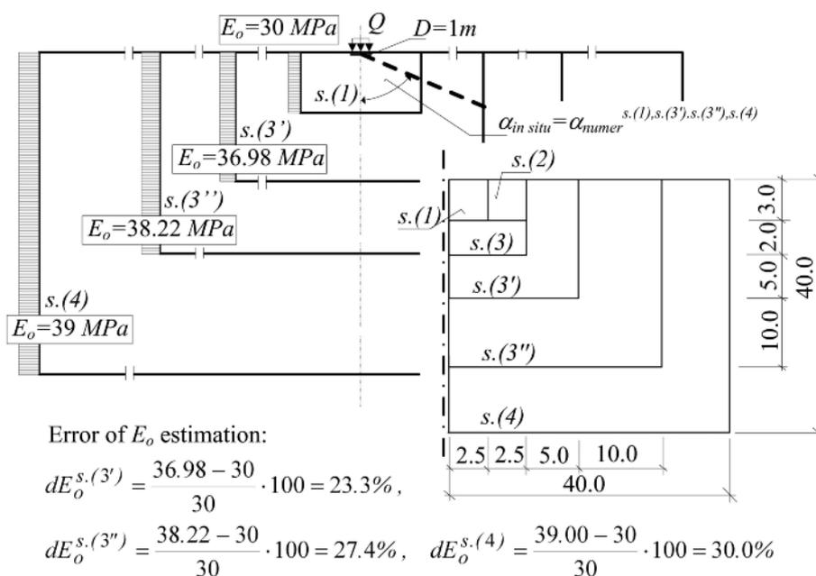
Figure 4. Ambiguity in the elastic model that arise during a basic task reconstruction
