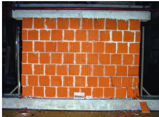
Figure 13. Falling-off of shells in compressed toes of the specimen
