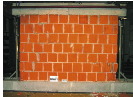
Figure 8. Disintegration of compressed toes in first load cycles
