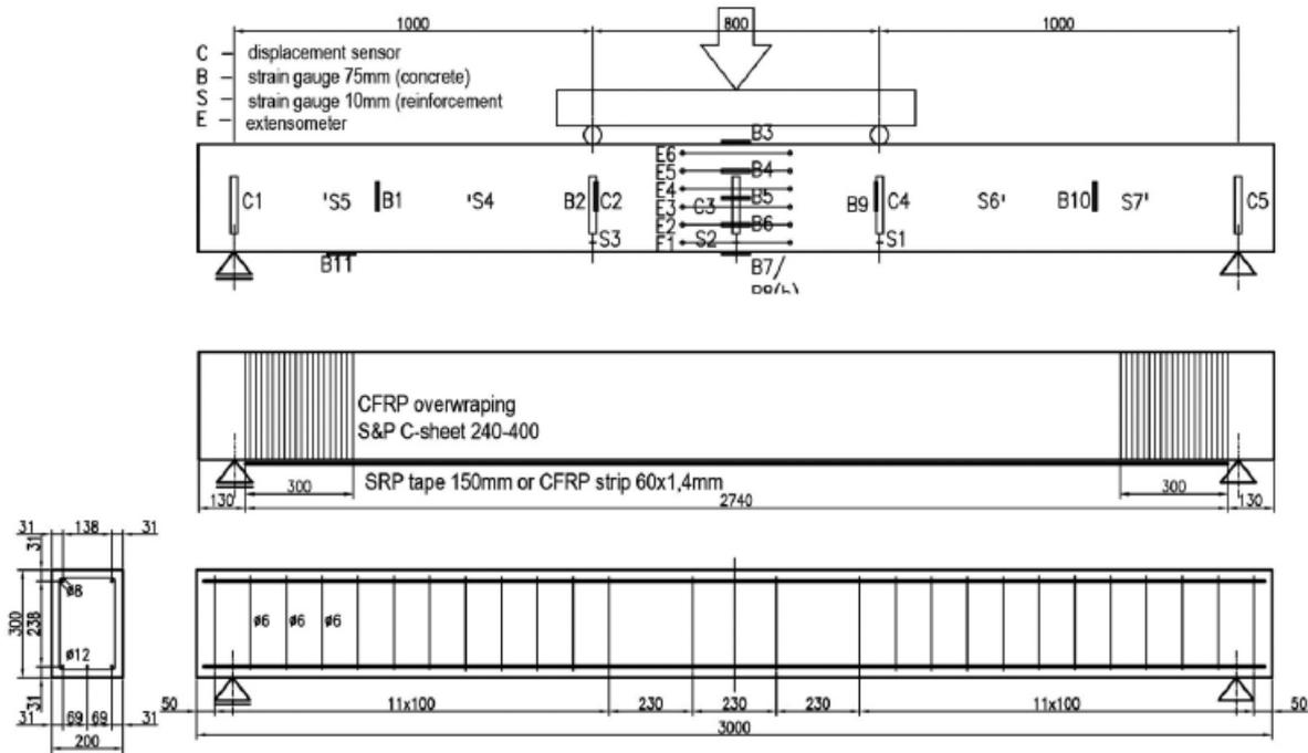
Figure 3. Details of the specimens (test scheme, reinforcement)
