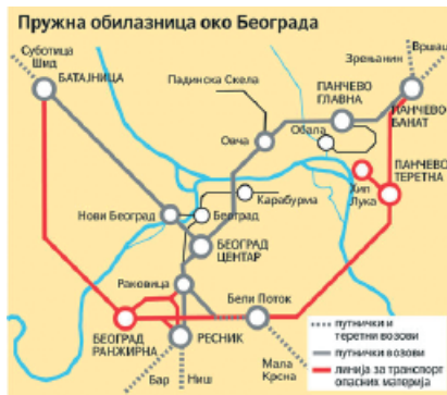
Figure 14 and 15. Belgrade Y (Metro Beograd) (existing) and Railways Half Ring network (grey – existing passengers’ and cargo railroads; red – planned for hazardous transports only)
