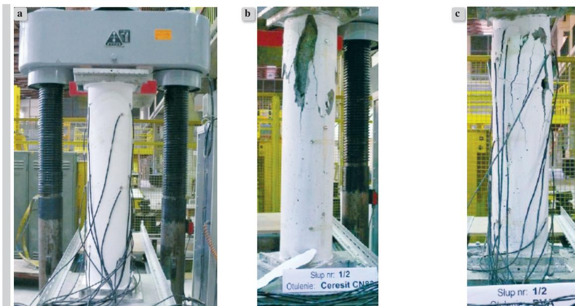
**Figure 7.** Tests of columns: a) set-up, b) failure mode with cement mortar cover, c) failure mode with PVA strengthening
