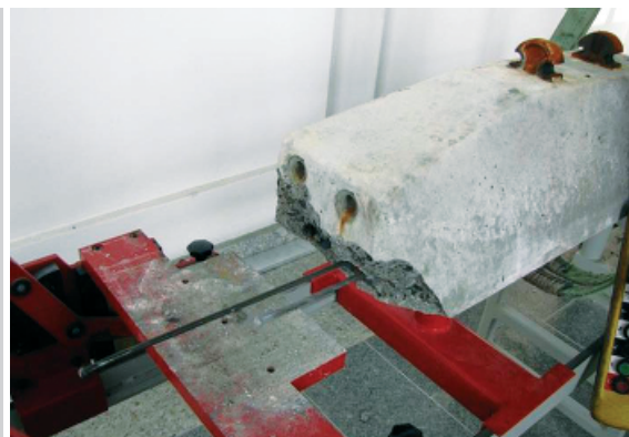
Figure 15. Failure of sleeper no. A-83/2b in static test
