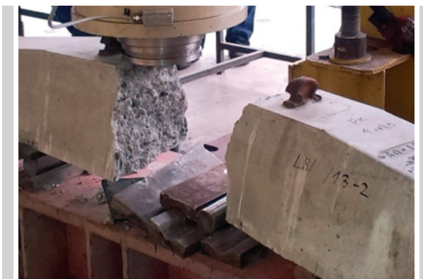
Figure 11. Failure of sleeper no. C-94/1 in fatigue test
