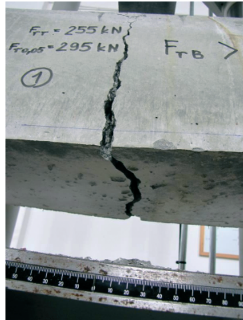
Figure 12. Failure of sleeper no. A-94/1 in static test
