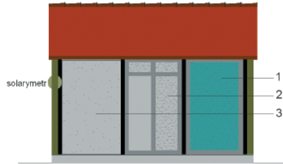
Figure 3. View of testing stand in the Faculty of Building Processes: 1 – partition with slab “okalux” 2 – partition with transparent insulation, 3 – analysed multilayer partition insulated in the first part with solid material and in the second part with perforated material
