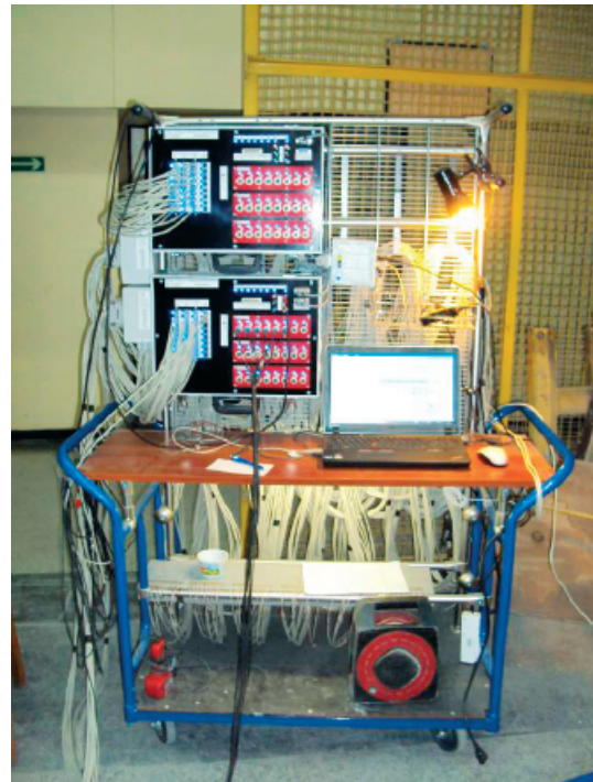
Figure 3. 128-channel signal converter with MLAB 32 software
