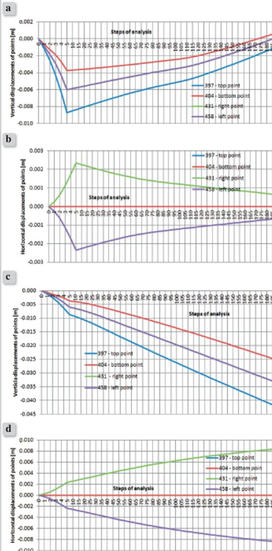
**Figure 4.** Diagrams of displacements of the main points of PVC-U pipe: a) vertical displacements – the effect of horizontal deformations of compressive character, b) horizontal displacements – the effect of horizontal deformations of compressive character, c) vertical displacements – the effect of horizontal deformations of tensile character, d) horizontal displacements – the effect of horizontal deformations of tensile character
