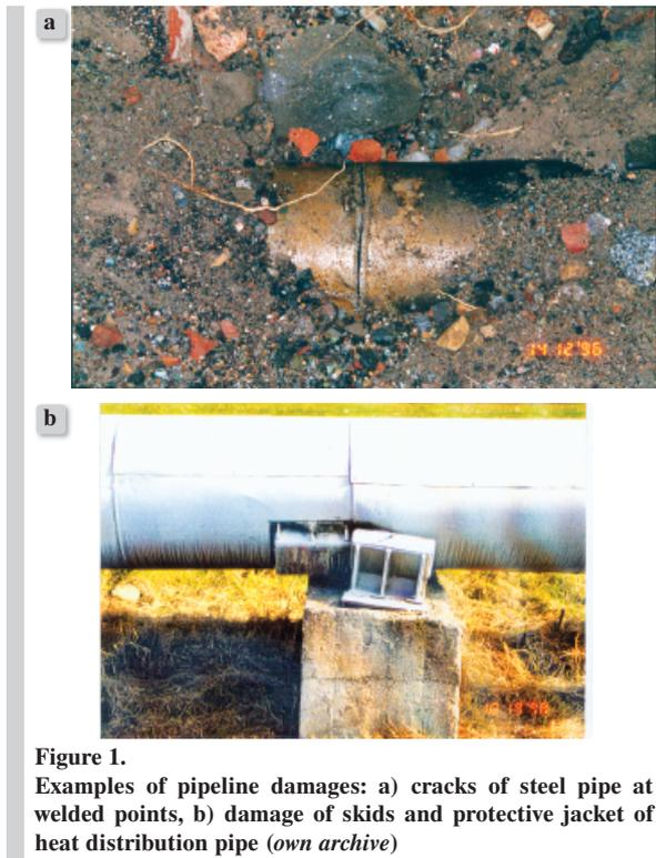
Figure 1. Examples of pipeline damages: a) cracks of steel pipe at welded points, b) damage of skids and protective jacket of heat distribution pipe (own archive)
