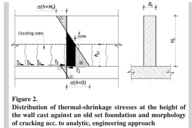
**Figure 2.** Distribution of thermal-shrinkage stresses at the height of the wall cast against an old set foundation and morphology of cracking acc. to analytic, engineering approach
