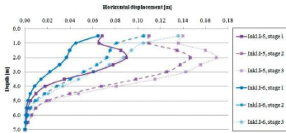
Figure 12. Horizontal displacements for I-5 and I-6 inclinometers
