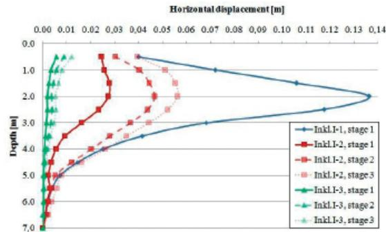
Figure 11. Horizontal displacements for I-1, I-2 and I-3 inclinometers
