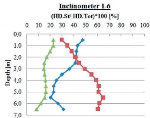
Figure 13. Percentage share of horizontal displacements at each stage in total displacements
