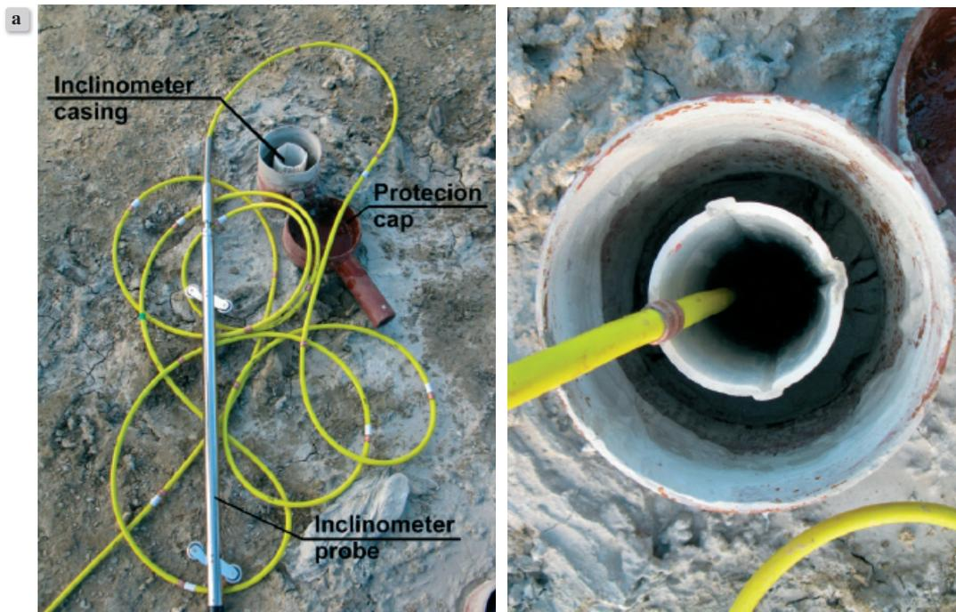
Figure 2. Set for inclinometer measurements: a) guide casing, cap, probe; b) guide casing details
