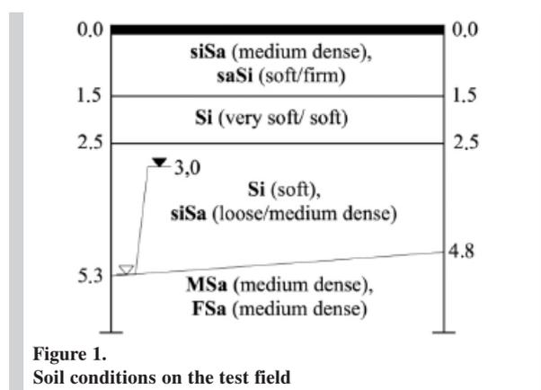
Figure 1. Soil conditions on the test field
