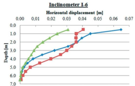
Figure 14. Horizontal displacement on each stage of column formation
