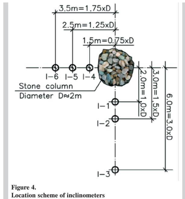
Figure 4. Location scheme of inclinometers
