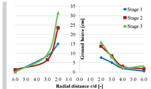
Figure 10. Ground uplift near the column
