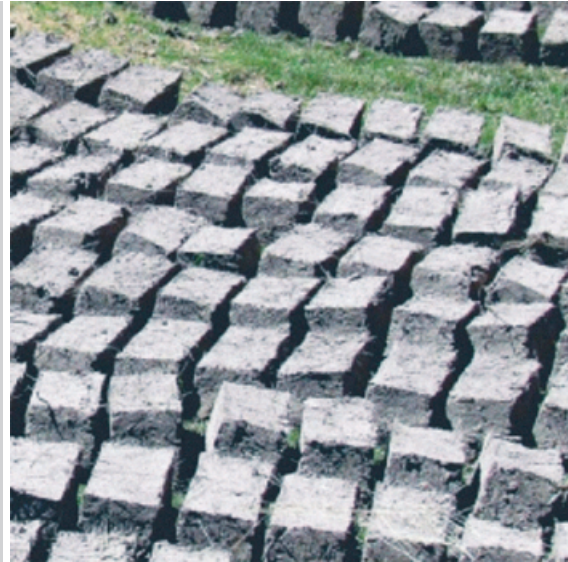
Figure 5. Adobe blocks (photo [5])
