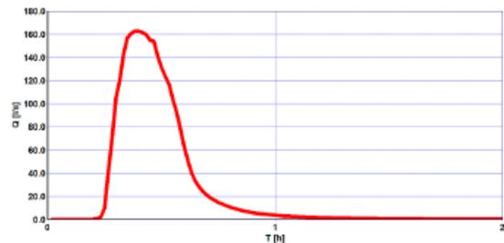
Figure 3. Drainage system discharge hydrogram
