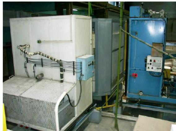
The “sun” chamber gives radiation in the spectral range close to natural one. Visible radiation in the range of wavelength  $400 \div 700\text{nm}$  allows the system of 20 metal halide lamps with power of 8kW generating temperature up to  $+75^\circ\text{C}$ . An additional system of ultraviolet radiants with wavelength of 185 and 255 nm imitates UV radiation.
