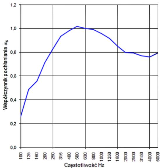
Figure 8. Sound absorption after 150 cycles of aging [28]
