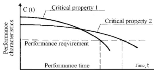
Figure 10. The principle of determining the performance time acc. to BS ISO 15686-2
