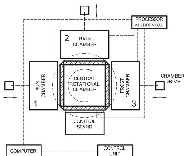
Figure 2. Position to simulate aging processes, schedule and view from the side of "rain" and "frost" chamber [21]
