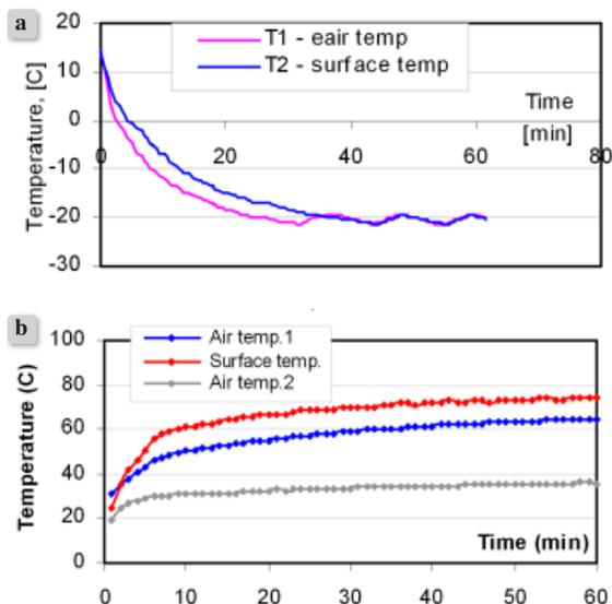
Figure 4. a. Characteristics of the chilling kinetics in the “frost” chamber [21] b. Characteristics of heating kinetics in the “sun” chamber [21]
