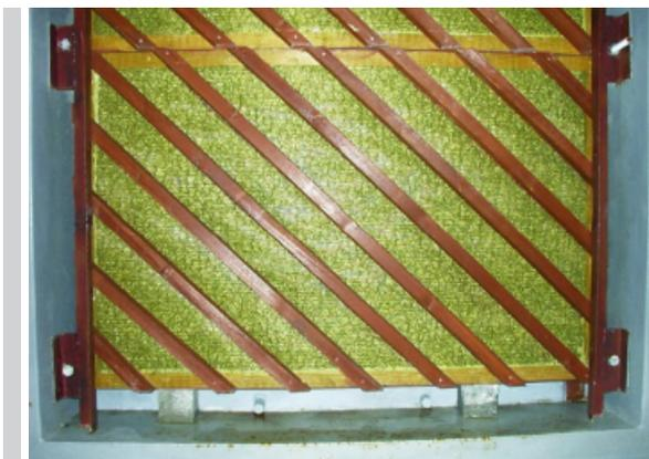
Figure 7. The view of acoustic panel in aging chamber [28]
