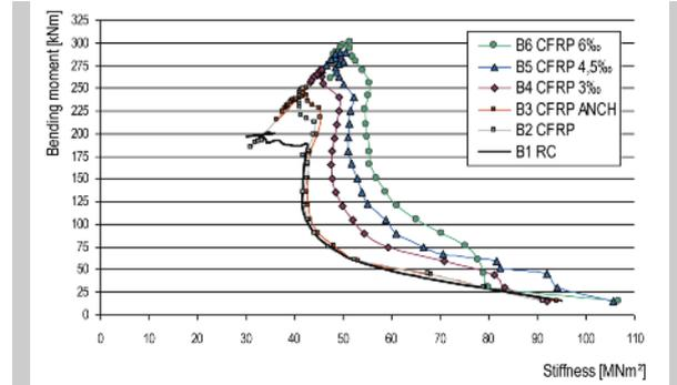
Figure 9. Load versus stiffness of tested beams
