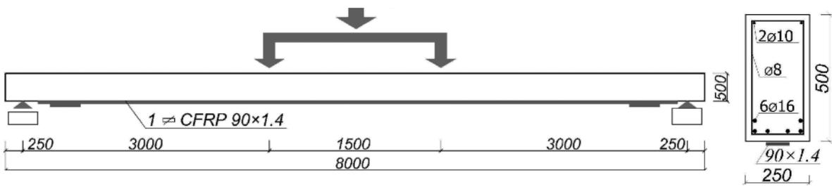
Figure 1. Dimensions, static schema and reinforcement of the beams in tests
