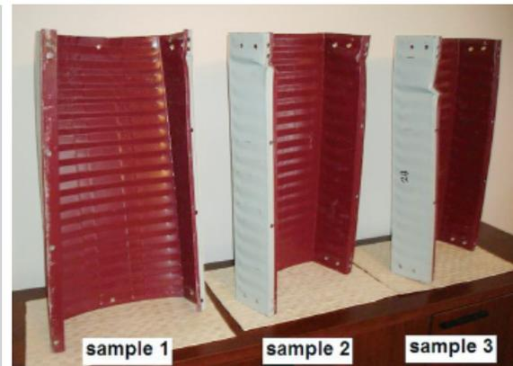
Figure 38. Eccentrically compressed curved panels with flat lips in compression
