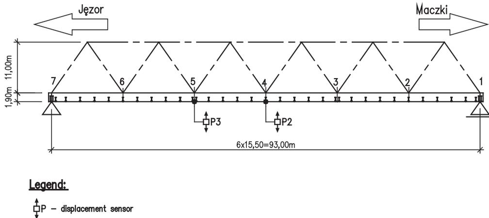
Figure 3. Inductive displacement sensors locations
