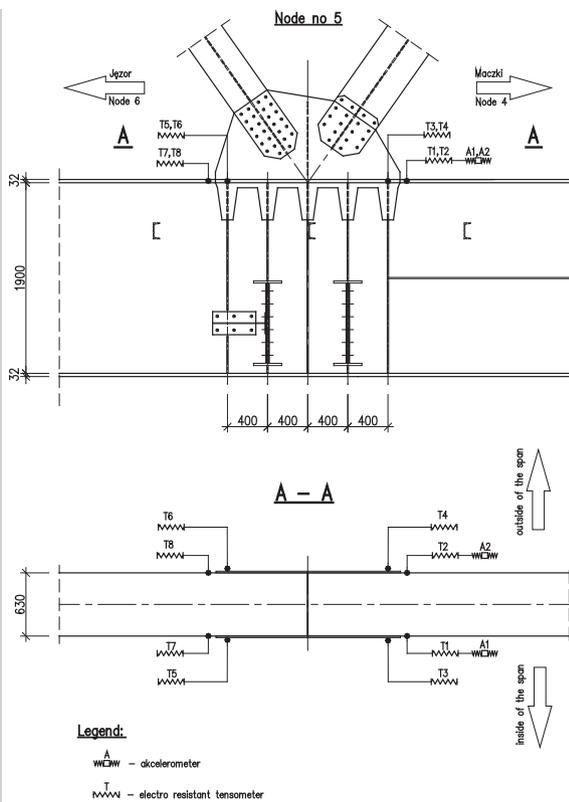
Figure 4. Electro resistant tensometers (T) and accelerometers (A)
