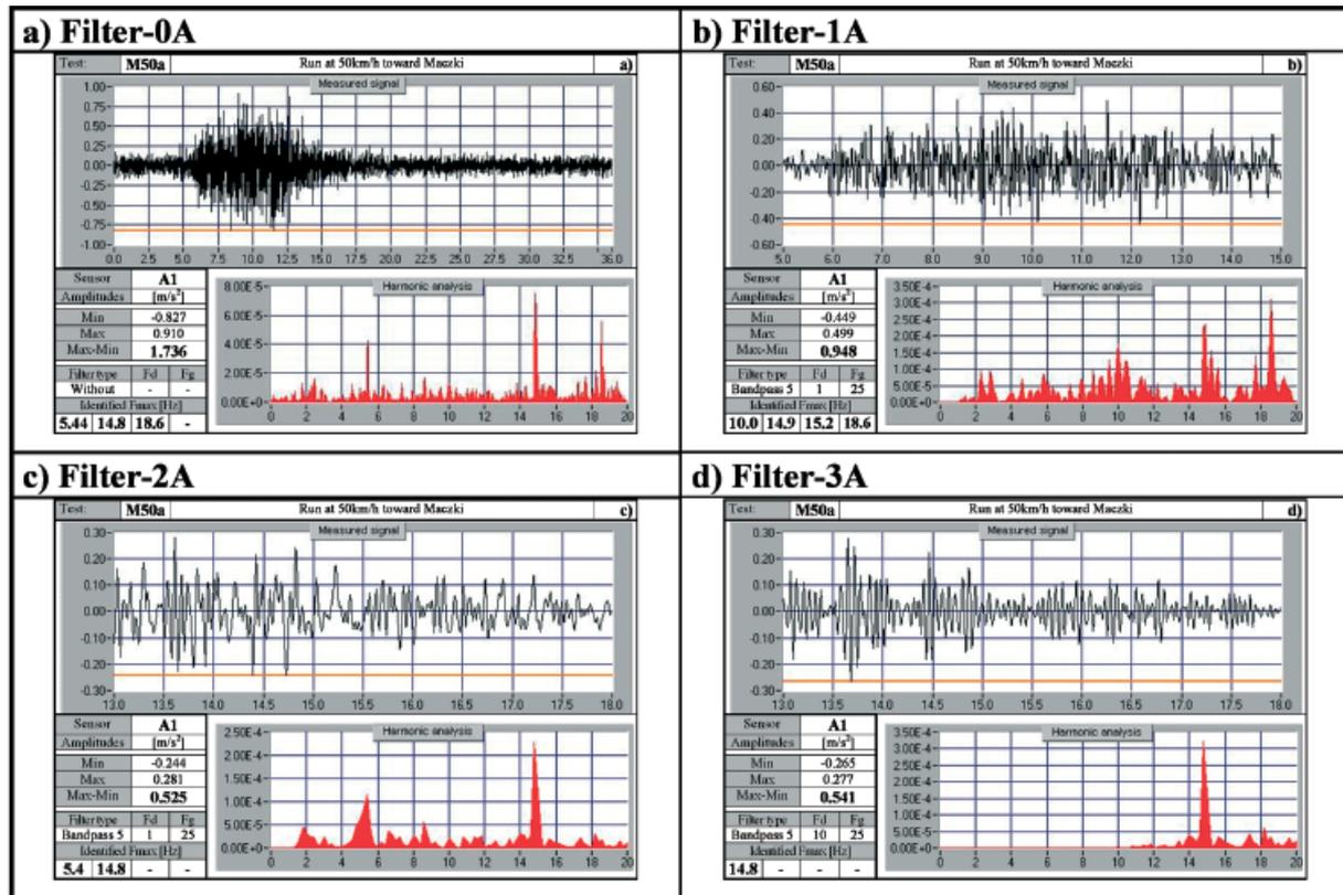
Figure 7. Accelerometer A1. Run at 50km/h toward Maczki: a) Filter 0A, b) Filter 1A, c) Filter 2A, d) Filter 3A
