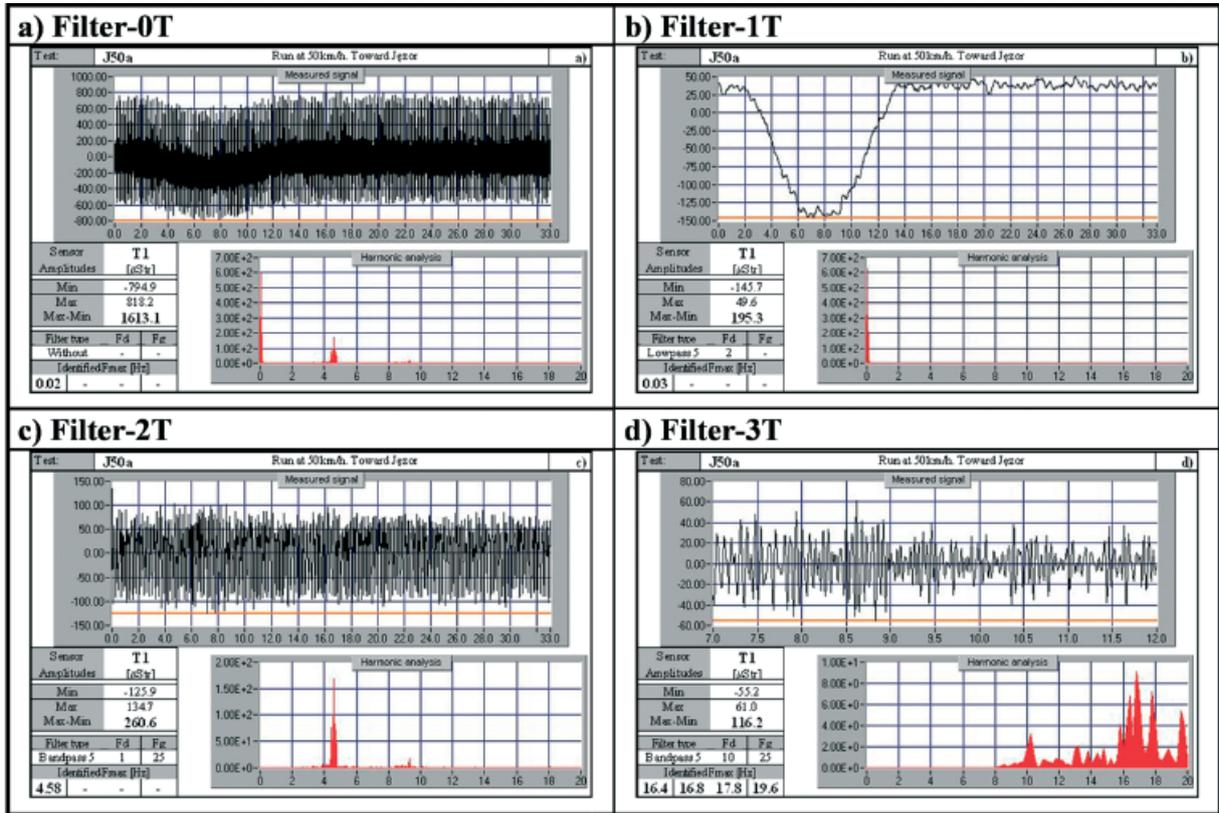
Figure 9. Electro resistant tensometer T3. Run at 50km/h. Toward Jęzor: a) Filter 0T, b) Filter 1T, c) Filter 2T, d) Filter 3T
