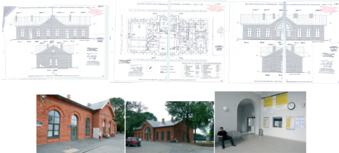
Figure 7. Documentation for the renovation of Pabianice railway station and photographs of the present state of the station building [8]
