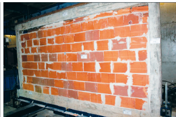
Figure 22. Crack pattern after out-of-plane test
