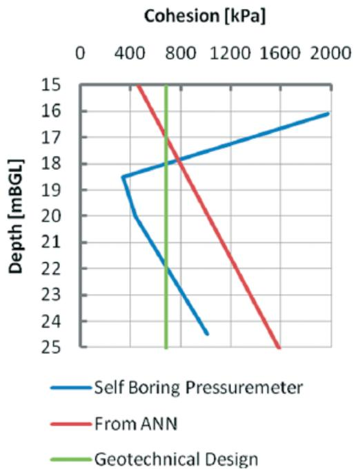
Figure 12. Comparison of cohesion obtained from different sources [1]
