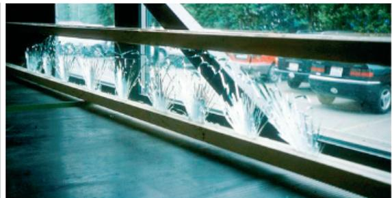
Figure 13. A beam after failure presenting a typical fracture pattern for timber-glass hybrid beam with the web made of annealed float glass [10]
