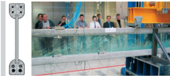
Figure 11. The cross-section of the glass-concrete beam and the specimen during test [9]
