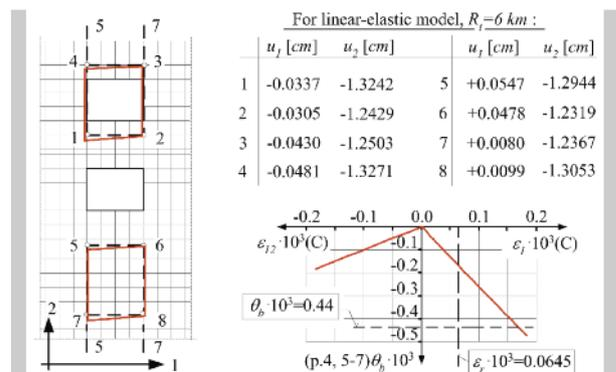
**Figure 7.** Deformations of two selected zones (from Fig. 5) and chart of strains in selected point C
