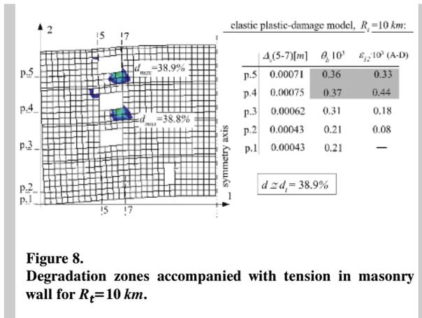
**Figure 8.** Degradation zones accompanied with tension in masonry wall for  $R_t=10\text{ km}$ .
