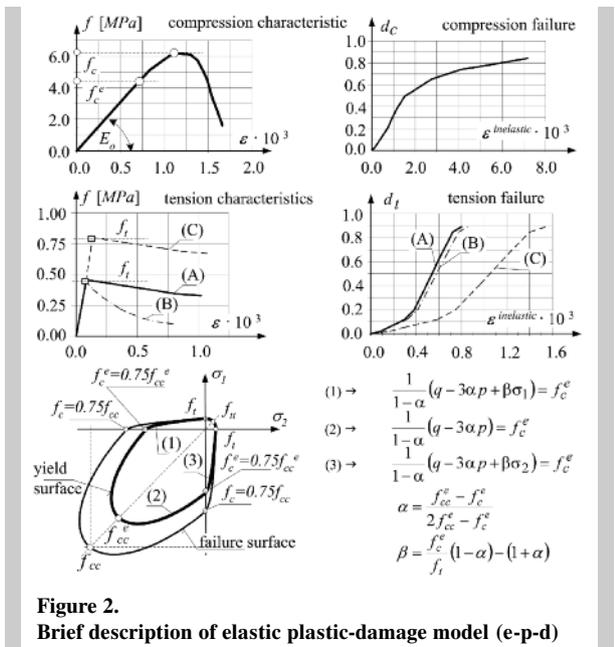
To make tracing of the following analyses possible Fig. 2 presents general description of the e-p-d model for masonry as:
