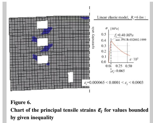
**Figure 6.** Chart of the principal tensile strains  $\epsilon_i$  for values bounded by given inequality
