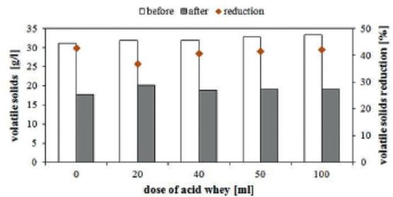
Figure 3. Volatile solids before and after co-digestion process
