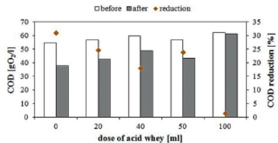
Figure 4. COD before and after co-digestion process
