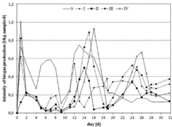
Figure 2. Intensity of biogas production rate during co-digestion
