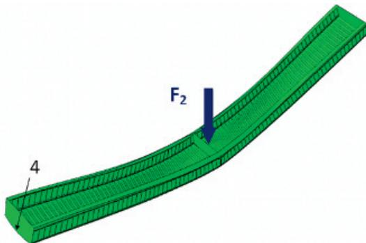
Figure 12. Deformed shape of FP2 model
