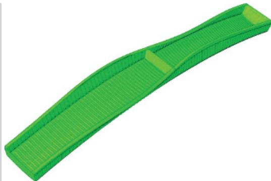
Figure 14. First, global (distortional) buckling mode
