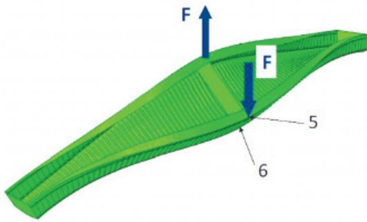
Figure 13. Torsional analysis of FP1 model
