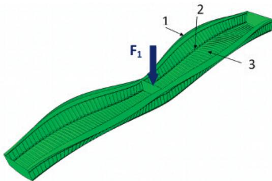
Figure 11. Deformed shape of FP1 model
