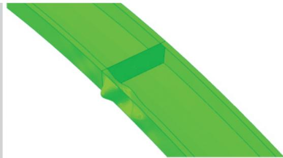
Figure 18. Local buckling mode of SP1
