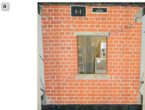
Figure A2. Final failure mechanisms for URM specimen: (a) Experimentally observed at \theta_{max} = +0.02 radian; (b) Theoretical prediction
