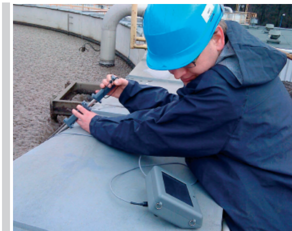
Figure 3. The respiratory activity measurement of the activated sludge with the use of the respirometer directly in the chamber of the activated sludge
