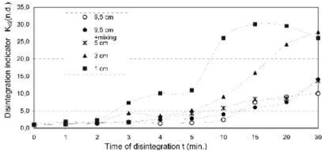
Figure 1. Influence of sludge layer height over the emitter on disintegration indicator  $K_{d2}$  for sludge KI ( $C_0 = 3.6\%$ ) and ultrasonic washer No 1 ( $f = 40$  kHz)
