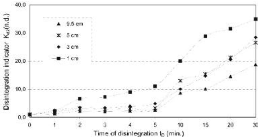
Figure 2. Influence of sludge layer height over the emitter on disintegration indicator  $K_{d2}$  for sludge KI ( $C_0 = 3.6\%$ ) and ultrasonic washer No 2 ( $f = 25$  kHz)
