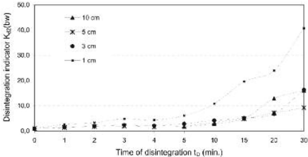
Figure 3. Influence of sludge layer height over the emitter on disintegration indicator  $K_{d2}$ , for sludge KII ( $C_0 = 3.5\%$ ) and ultrasonic washer No 4 ( $f = 22$  kHz)
