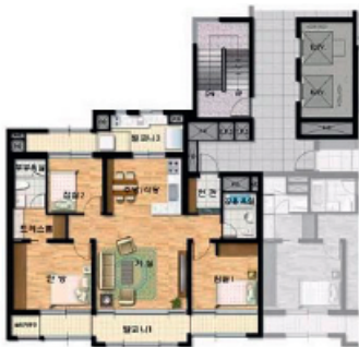
Figure 9. The floor plan of around 34 pyong (approximately 112 m 2 ) unit. Other size units have a generally similar arrangement, but only the number of rooms is different. (Source: Samsung Raemian webpages)
