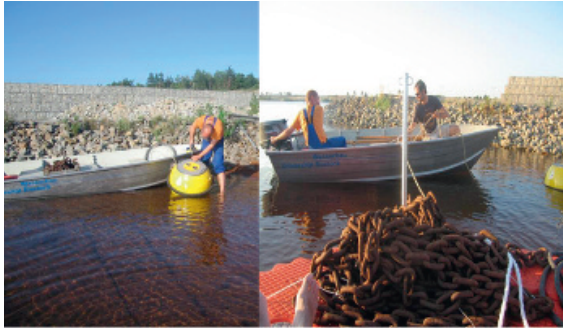
Figure 29. For installing of the measuring buoy in the lake of a former opencast lignite mine a long and heavy anchor chain is necessary
