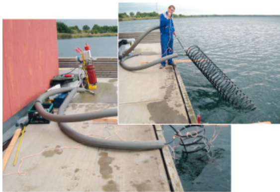
Figure 14. Experiments with regard to the investigation of an optimisation of the heat exchange in surrounding water
